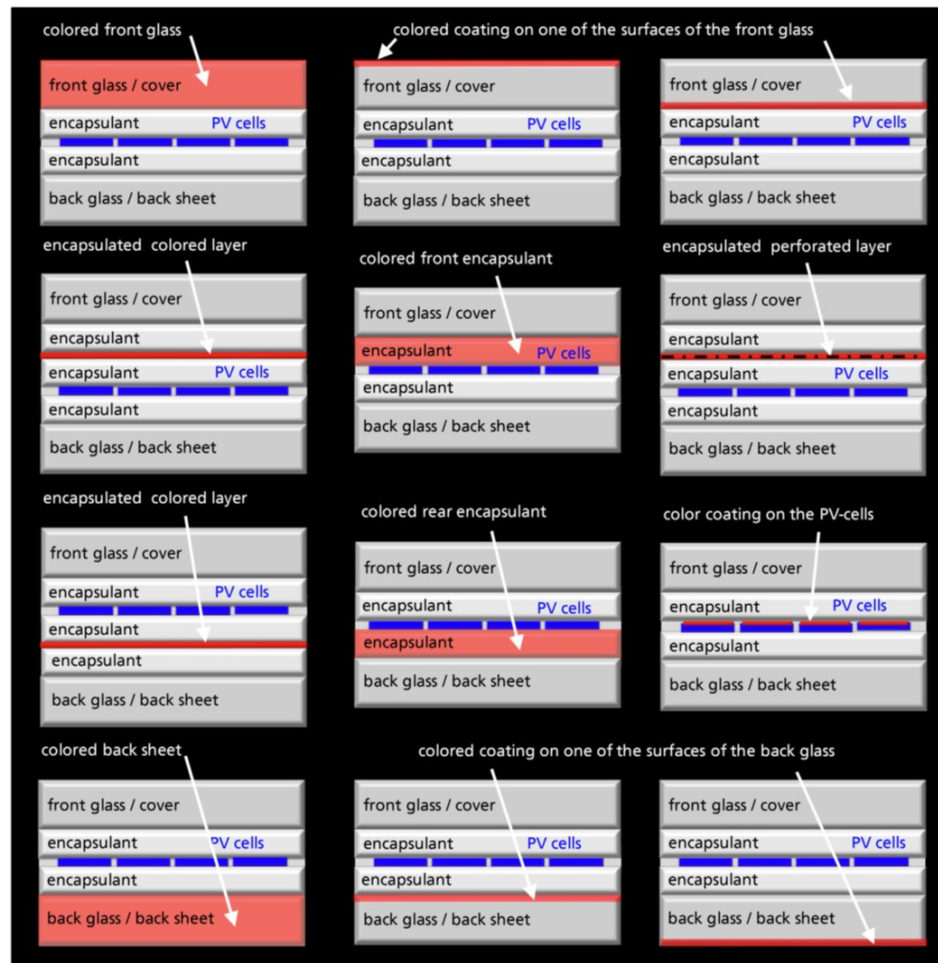
Figure 2.15: Colored PV module strategies, with technical design options sorted from outside to inside, with the outer layer on top. The colored layer or surface is highlighted in red. Reproduced from [66].
