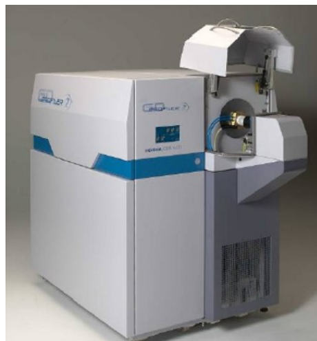
Figure 2.3: A photograph of the GD Profiler 2 by HORIBA Scientific. It is an RF-GDOES instrument, shown here with the sample compartment cover open [24].
