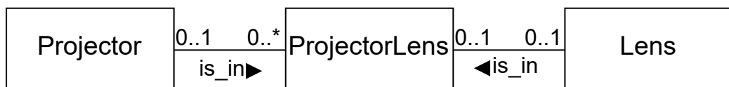
Figure 17: Relationship of tables in projector/lens database. A more detailed figure can be seen in the appendix A, Figure 41.
