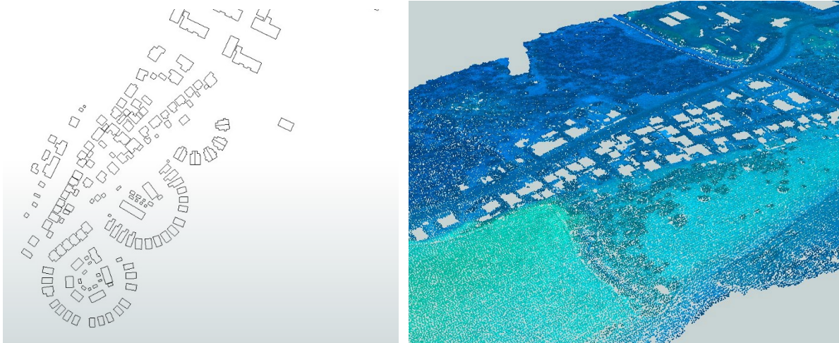
Figure 5. Input data for 3D model generation in FME software: 2D footprint file (left) and point cloud Lidar file with filtered out points classified as Ground based (right).
