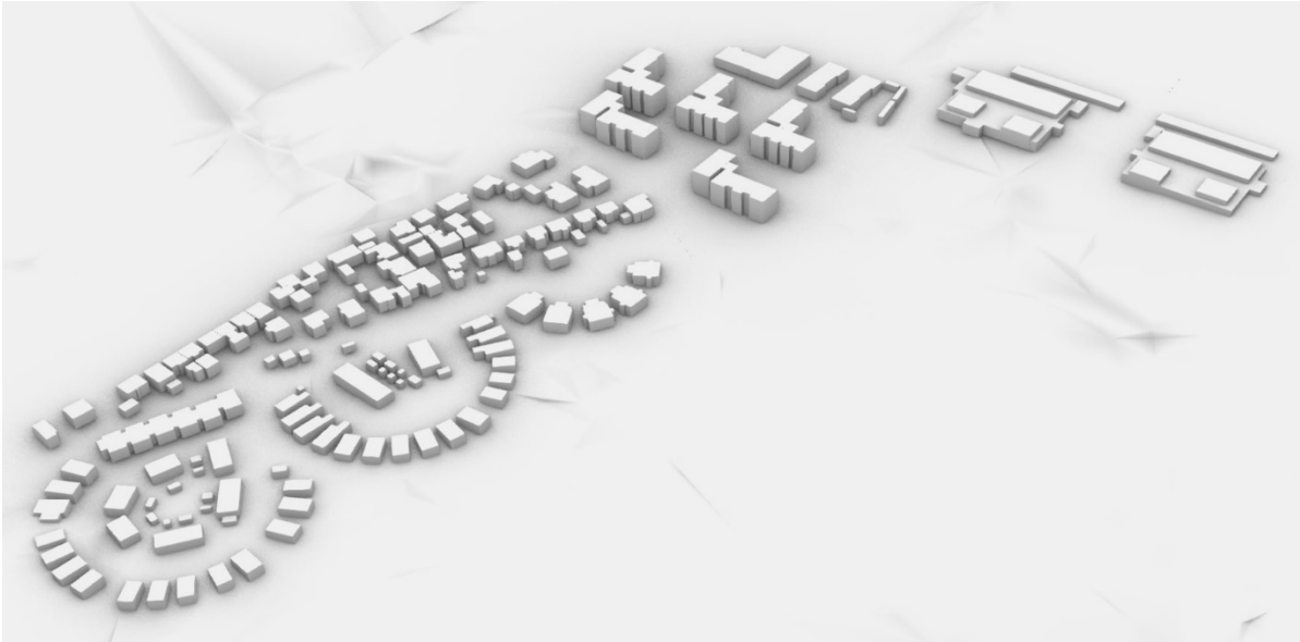
Figure 17. The view of the 3D model for existing buildings in the neighborhood generated with 3dfier software.
