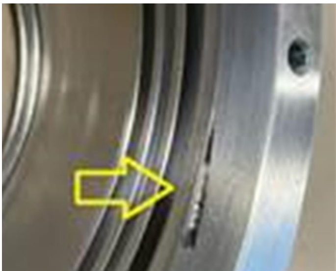
Picture 1: Surface scratch on a part (J. Elnaes 2023, personal communication, 15 May).
