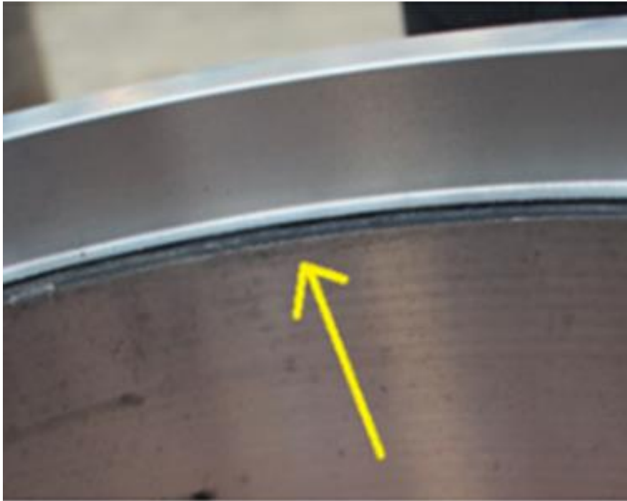
Picture 2: Lack of material in part (J. Elnaes 2023, personal communication, 15 May).
