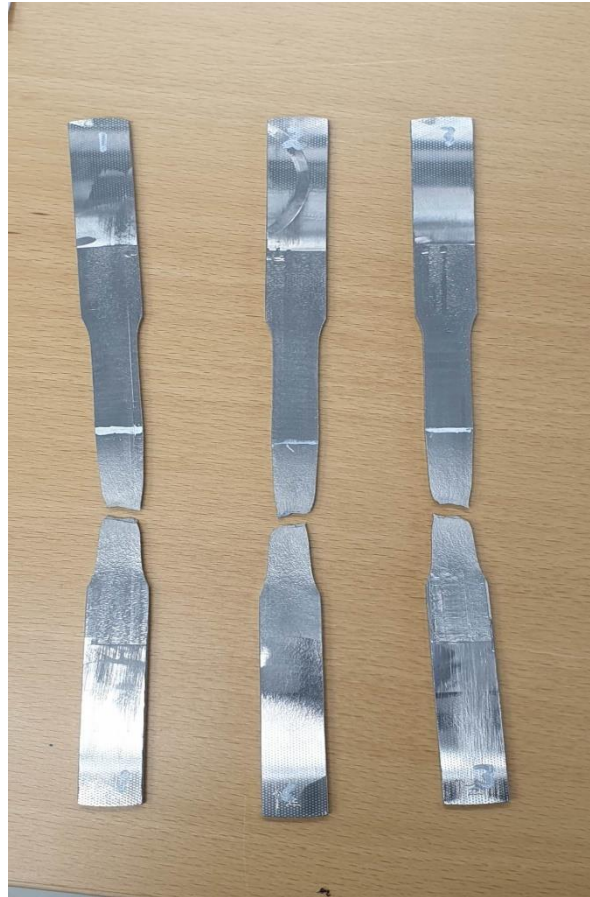
Picture 25: All specimens after fracture. Note the necking in all samples.
