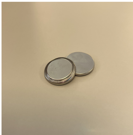
Figure 3.3: Fully assembled coin cells.
