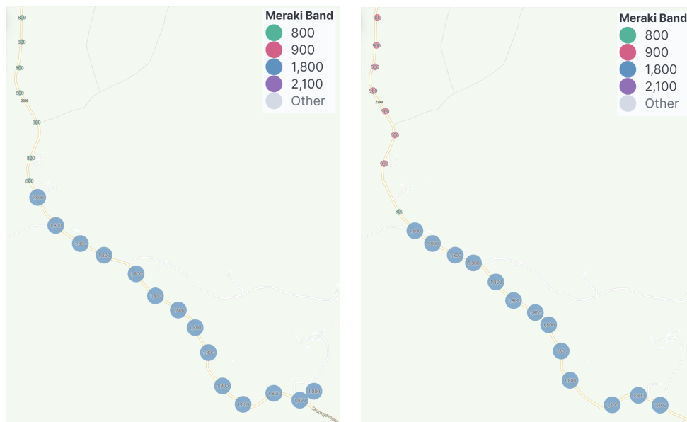
(a) Frequency bands used on the first round driving north (b) Frequency bands used on the third round driving north
