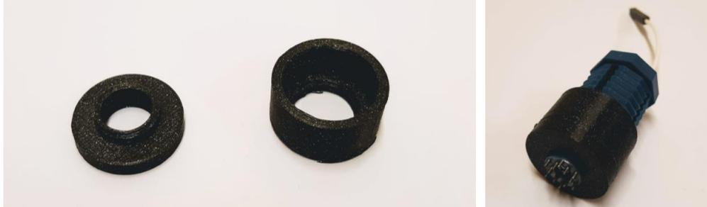
**Figure 2. First iteration prototype. Bottom and top part of the adapter (left). Assembled adapter attached to the dry electrode (right).**
