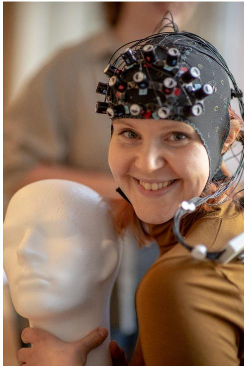
**Figure 4 fNIRS headgear. Sources (marked in red) and detectors (marked in blue) are arranged into a montage placed on the prefrontal cortex. [Photo taken by Pasi Aalto]**
