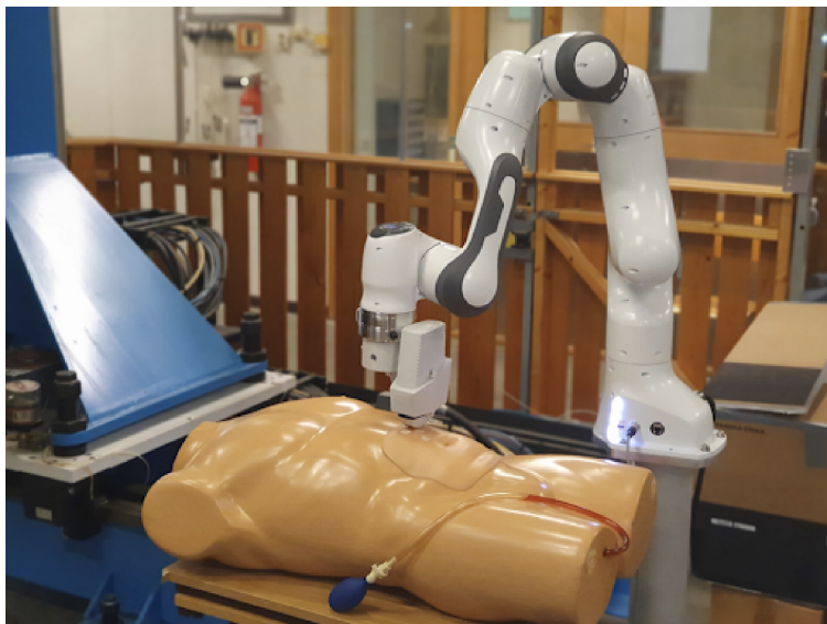
Figure 1.1: Example laboratory set-up we use for a robotic ultrasound on a human dummy.
