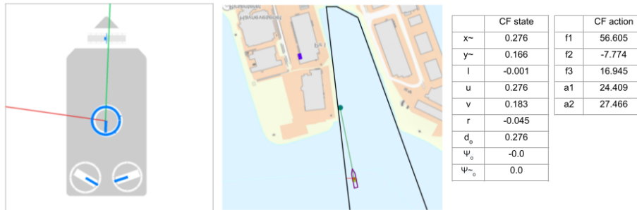
Fig. 4. The table shows the counterfactual explanation by stating how much the state and the action would change in the counterfactual example for the situation given by the vessels point of view(top left) and how the vessel is situated in the harbour (right).
