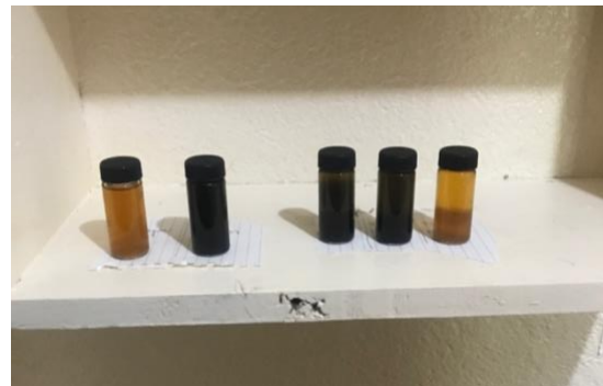
Figure 3.8: Measurements of hydrogen-sulphide producing bacteria showing both positive tests (black colour or black precipitate) and negative samples (yellow colour).
