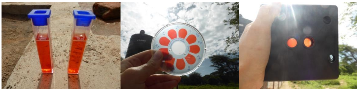
Figure 3.7: Measurement of fluoride concentrations showing the mixed samples (left), the coloured disc (middle), and the comparison of sample and disc (right).
