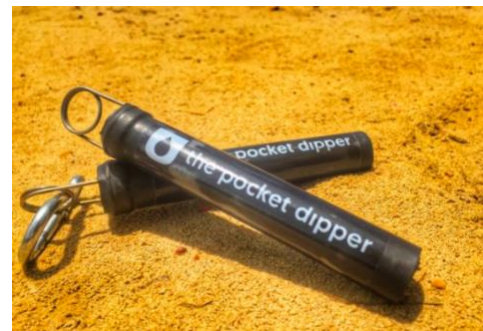
Figure 3.4: Pocket dipper to measure groundwater levels in the wells (Groundwater Relief, 2020).
