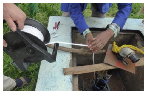
Figure 3.5: Measuring tape with the light signal on the other side of the black casing.
