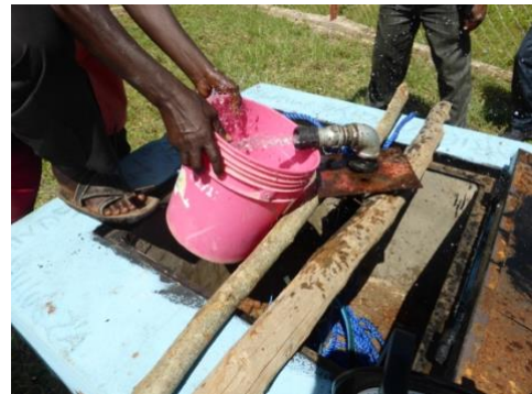
Figure 3.3: Bucket testing to measure flow rate from the wells.
