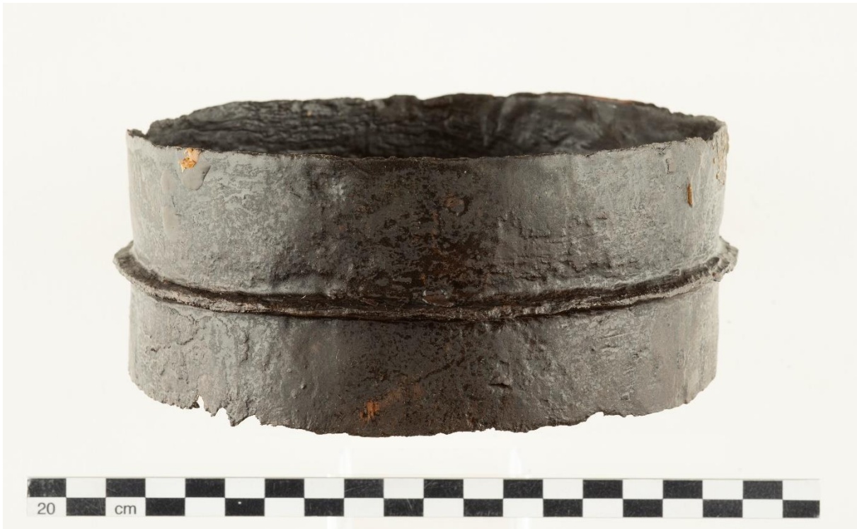
Figure 26: Iron ring for connecting two hollowed wooden logs in the 1777 piped system in Trondheim (N25042, collections online). Photo: Ole-Aleksander Ulvik. © NTNU Museum of Science.
