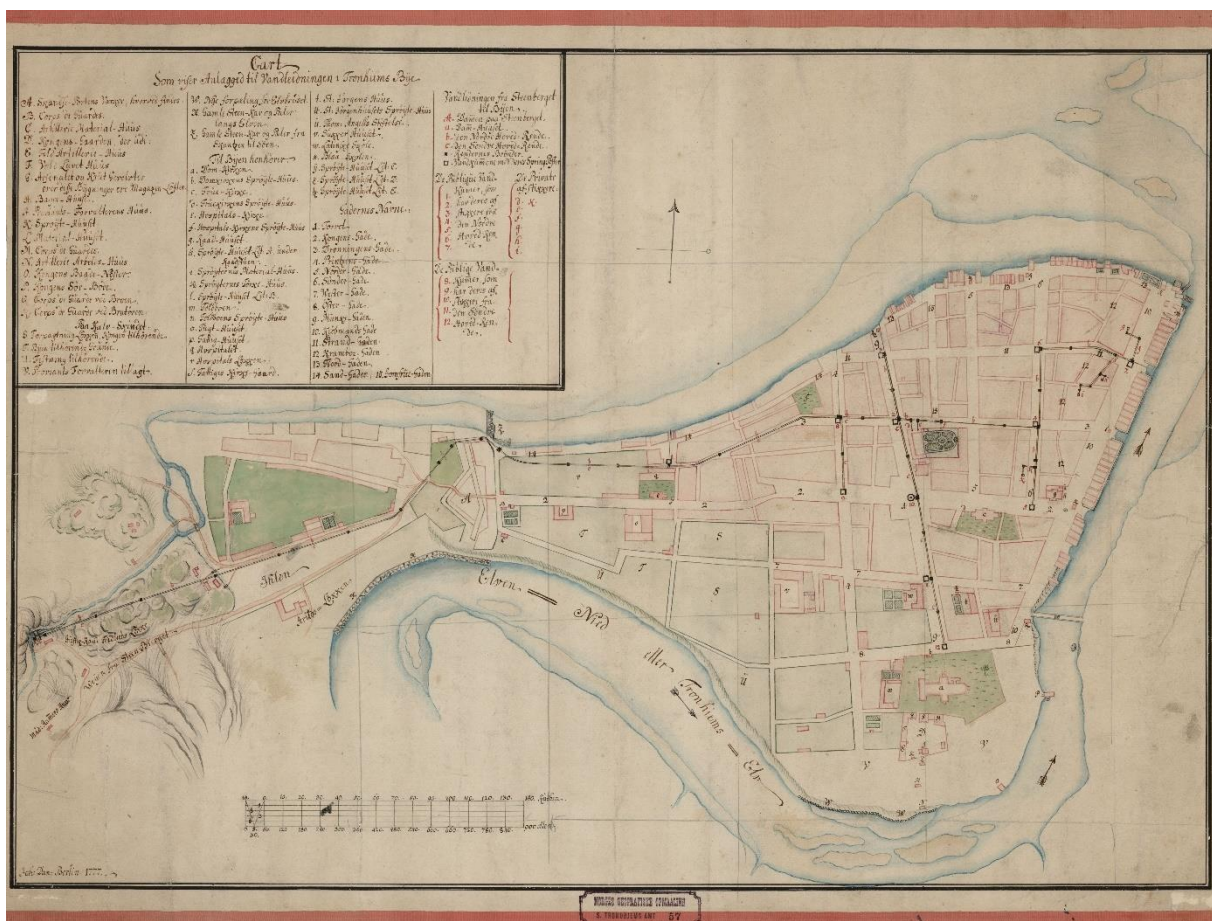
Figure 19: The original 1777 water pipes (black lines) and water pumps (black squares) in Trondheim, both public and private branches, by Johan Daniel Berlin. ©Kartverket.no (Berlin, 1777).
