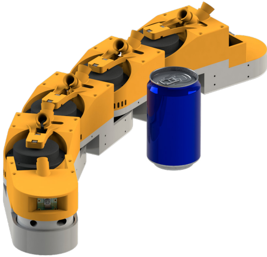
Fig. 4. A digital render of a 5-link Boa snake robot, with a soda can for scale reference.
