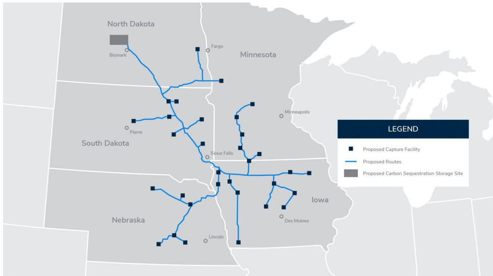
Figure 2.10: Illustration of the planned pipeline network in the Summit Carbon Solutions project (Summit Carbon Solutions 2022).
