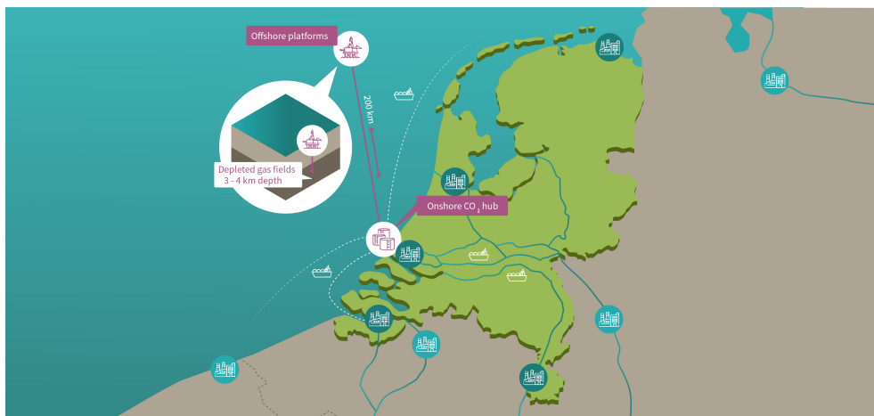
Figure 2.9: The transportation network in the dutch Aramis project with emission sources, collecting CO 2 hub in Rotterdam and pipeline transportation to storage in a depleted oil and gas field in the North Sea (Aramis 2022)
