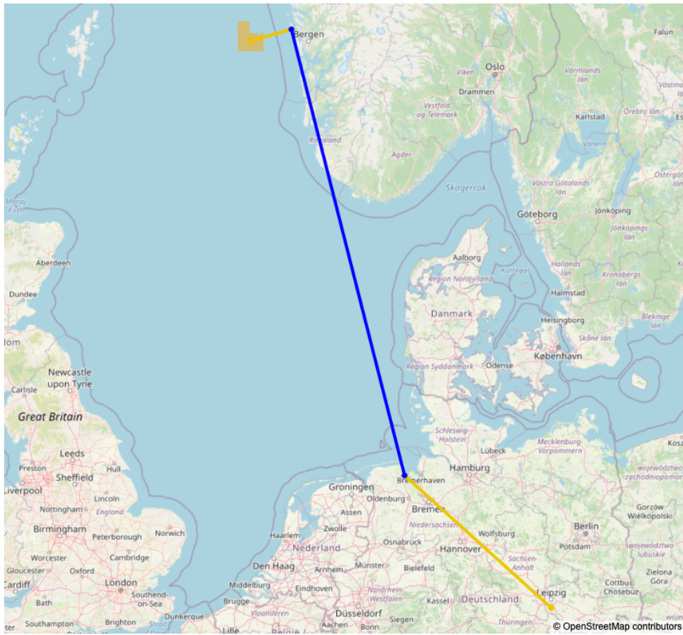
Figure 7.3: Optimal transportation network for scenario S5. The blue line represents ship connections between the ports, while the yellow lines represent pipeline connections with a yearly flow of 5 Mt.
