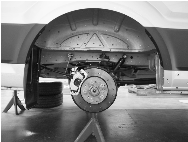
Figure D.1: The scanning process involves the placement of many randomly placed reference markers on the surfaces that are to be scanned. (Photo: NTNU/Sebastian Reymert)
