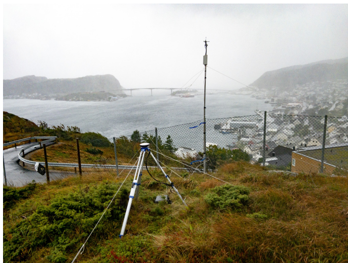
Figure 6.8: The base station in operation over Måløy with the bridge in the background. The GNSS receiver antenna is mounted on the tripod (left) and the radio modem and antenna on top of a telescopic mast (right). (Photo: NTNU/Sebastian Reymert)
