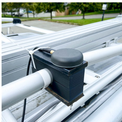
(a) Detail of GNSS receiver mounting
