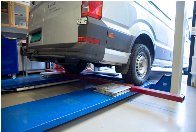
Figure C.1: The test vehicle being backed into place on the end of an hydraulic vehicle lift. Each of the rear wheels was resting on a load cell when measurements of rear axle weight and angle were taken to estimate the height of the CG. (Photo: NTNU/Sebastian Reymert)
