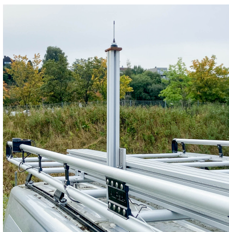
(b) Detail of radio antenna mounting
