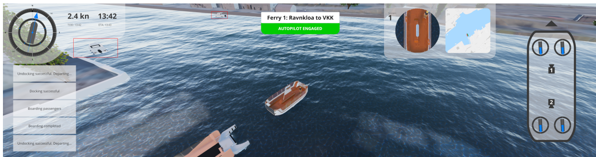
Figure 10: Autoferry Gemini, a simulator for testing and developing HMI for the operator
