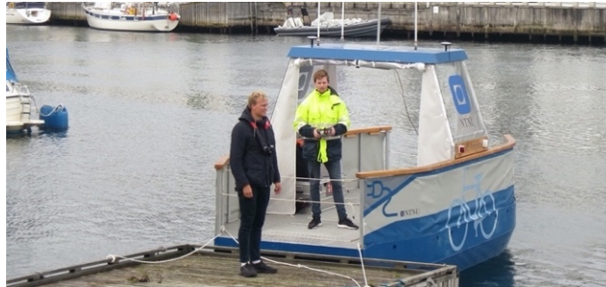
Figure 7: The all-electric urban autonomous passenger ferry milliAmpere1 (Photo: Egil Eide)
