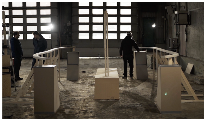
Figure 11: The MRLab is a mixed reality lab to test different physical layouts and functionality of urban autonomous passenger ferries in virtual reality (Photo: Nicholas Lund).
