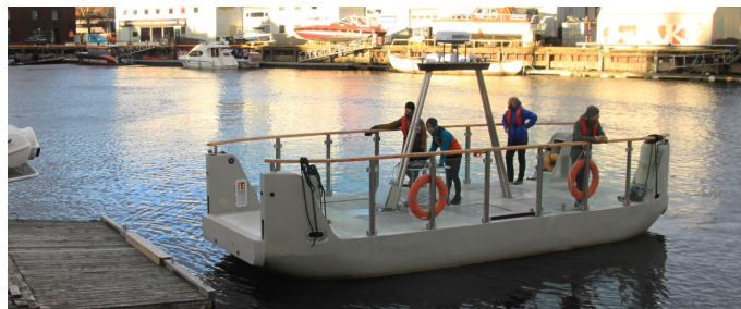
Figure 8: The all-electric urban autonomous passenger ferry milliAmpere2 (Photo: Egil Eide)
