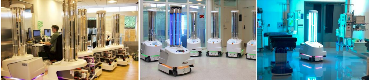
Figure 12 Indoor disinfecting robot UVD, consisting of a mobile base equipped with multiple LIDAR sensors and an array of UV lamps mounted on top. Credit: UVD Robots.
