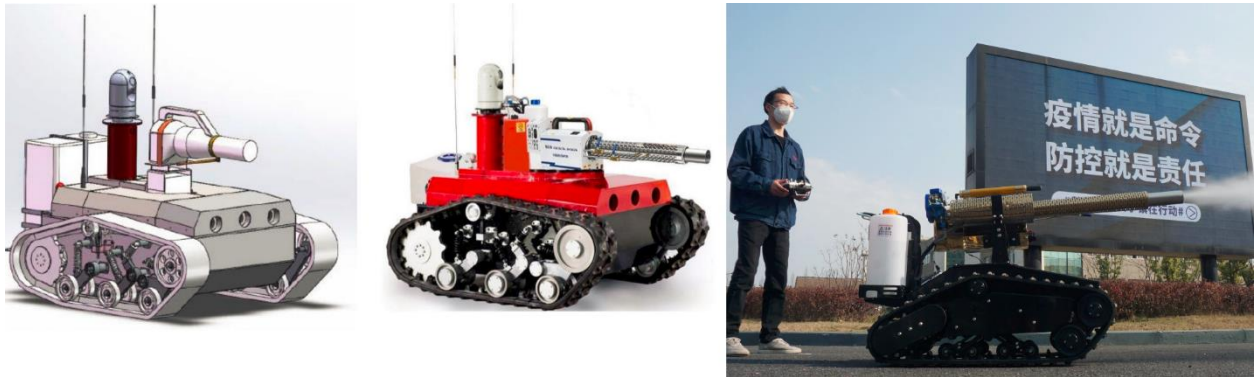
Figure 11 Outdoor disinfecting robot from Siemens, the Chinese company Aucma working in the joint laboratory for robot applications in Qingdao. The robot was designed using CAD and the actual system was built in just a week. Credit: SIPA Asia
