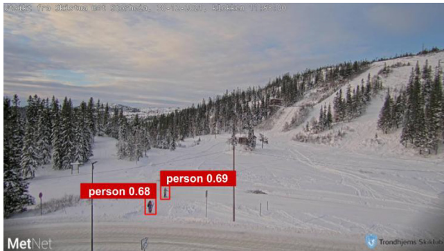
Fig. 2. Two persons detected by the YOLO image recognition model with corresponding confidence.
