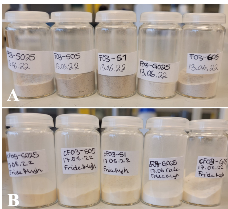
Figure 4.4: Images taken of the powder samples before (A) and after (B) calcination of the samples with synthesis A from experiment investigating addition order.
