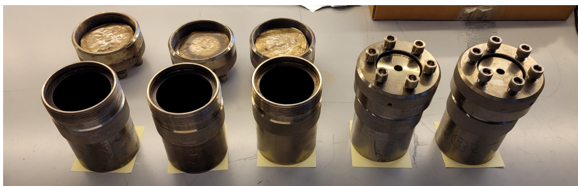
Figure 2.3: Autoclaves used for hydrothermal synthesis, where a Teflon-lined container containing the gel solution is sealed inside the stainless steel autoclave followed by crystallisation in the oven.
