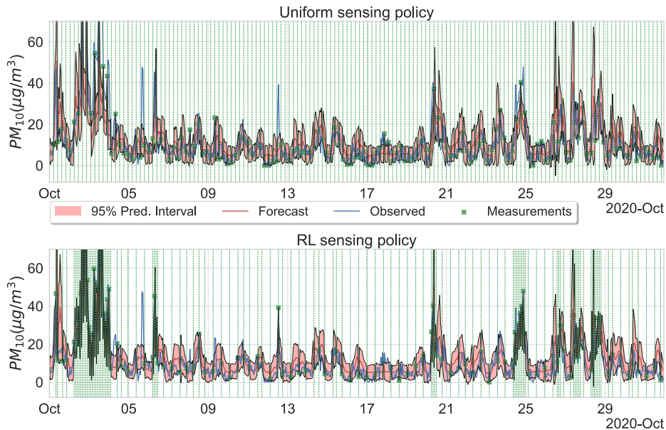
Figure 4.5: An example of a Bayesian neural network prediction model of the air quality over one month. The top model is fitted with measurements selected uniformly, while the bottom model is fitted with measurements selected using a deep reinforcement learning agent. The dotted, green vertical lines show the measurements’ time index. The learned policy detects and densely senses the air quality during periods when it is high, while the uniform policy spreads its measurements uniformly. (Adapted from figure V.61 in Paper V)
