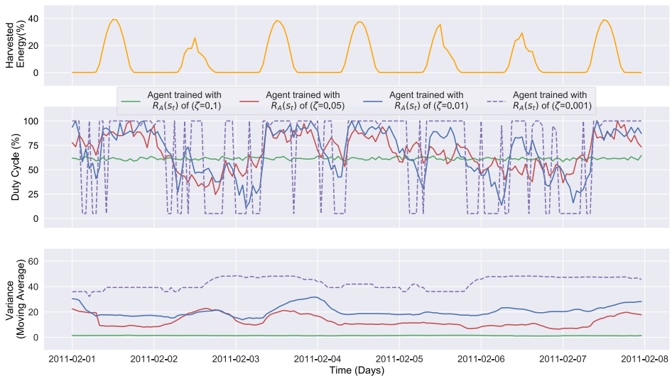
Figure I.7: Performance results over one week (Tokyo 2011) of four selected agents trained with different damping factors ( \zeta ) in their reward function R_A(t)
