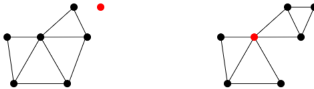
Figure 5.1: The triangular mesh is assumed to have no disconnected vertices, as in the left figure, and no parts only connected by a single vertex, such as the figure on the right.
