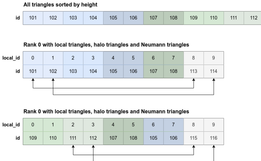
Figure 4.9: An example of how local ids are used when splitting triangles into groups. The triangles are first sorted by their vertical coordinates before they are split in two groups, colored with blue and green. The triangles that are at the border of the other group are marked with a darker color, and triangles at the edge that are missing a neighbor are marked with a lighter color. Rank 0 has the blue triangles in addition to the neighboring triangles, and rank 1 has the green triangles in addition to the neighboring triangles. Rank 0 and 1 also need to create mirror triangles, referred to as Neumann triangles and shown in Fig. 4.6, that border the triangles missing a neighbor. For rank 0, triangle 113 is a mirror of triangle 101, always containing the same data as its mirror. All triangles are given a local id starting from 0 which is only visible for its rank.
