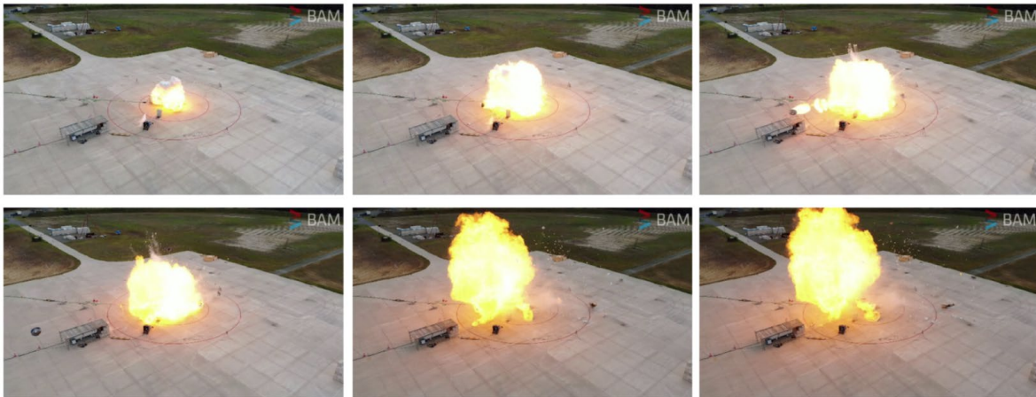
Figure 5: Fireball development after the failure of an MLI-insulated vessel positioned horizontally filled with liquified hydrogen as seen from a drone flying over the test pad.
