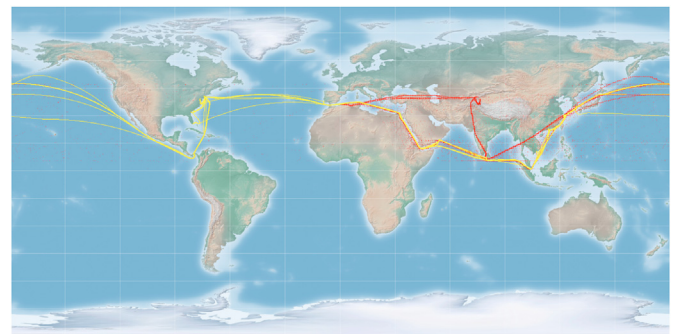
Fig. 16. Trajectory of vessel I.36 from class C.12. Red points refer to the CAMS registered coordinates and yellow refer to even-spaced AIS estimates of the interpolation methodology.
