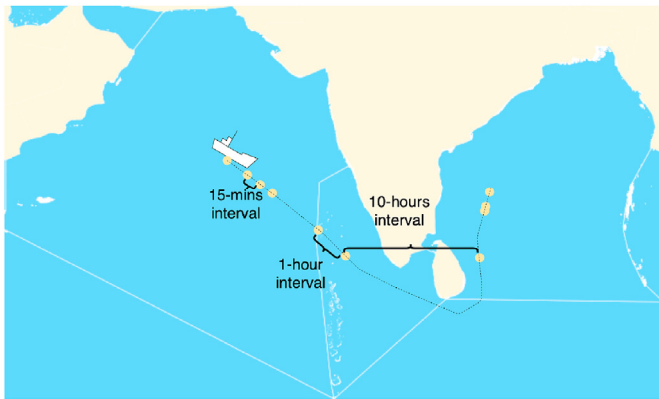
Fig. 13. Example of AIS coordinates with a long (10 h) gap included on the measurements. Yellow dots indicate the measurements and the black dashed line is considered to be the real trajectory of the vessel. (For interpretation of the references to colour in this figure legend, the reader is referred to the Web version of this article.)
