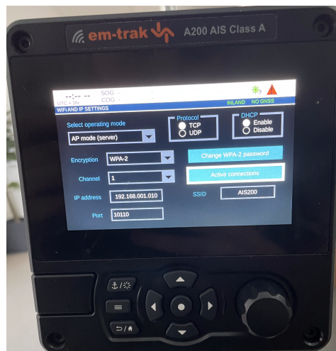
Figure 6. The Wi-Fi settings menu in A200.
