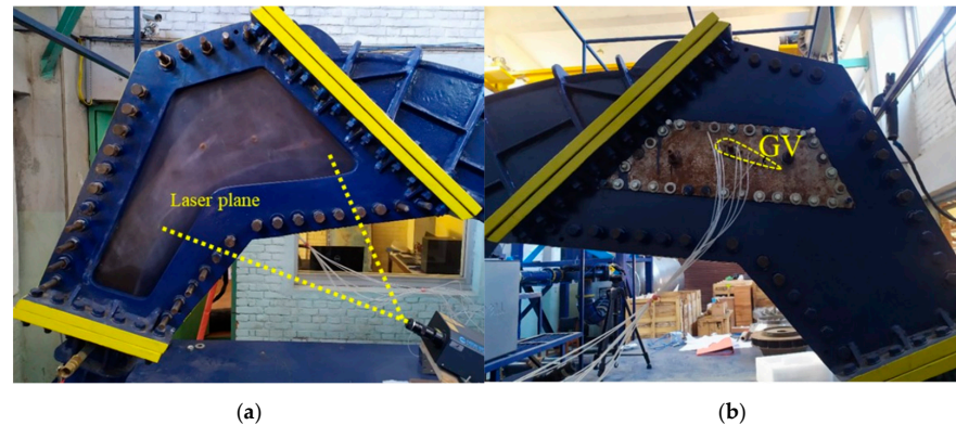
Figure 6. The three-GV test setup for experimental validation: (a) Experimental set up which shows the test section in the lab; (b) Locations of holes for tapping the value of pressure at GV.
