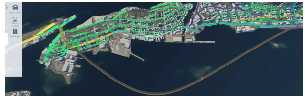
Fig. 7: Example of a case related to the inclusion of a new infrastructure. Two new links are added to the network: a bridge and a tunnel (highlighted in yellow).
