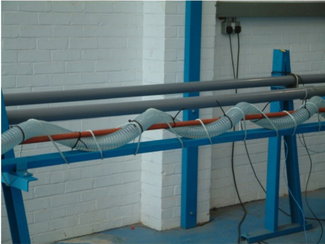
Figure 3-15: A photograph of the helical pipe suggested by (Adedigba, 2007).
