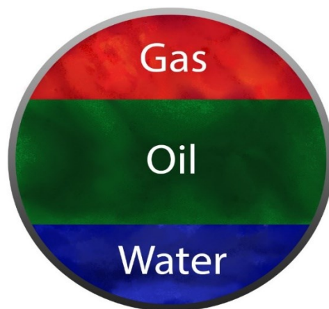
Figure 2-1: Three-phase flow pipe cross-section
