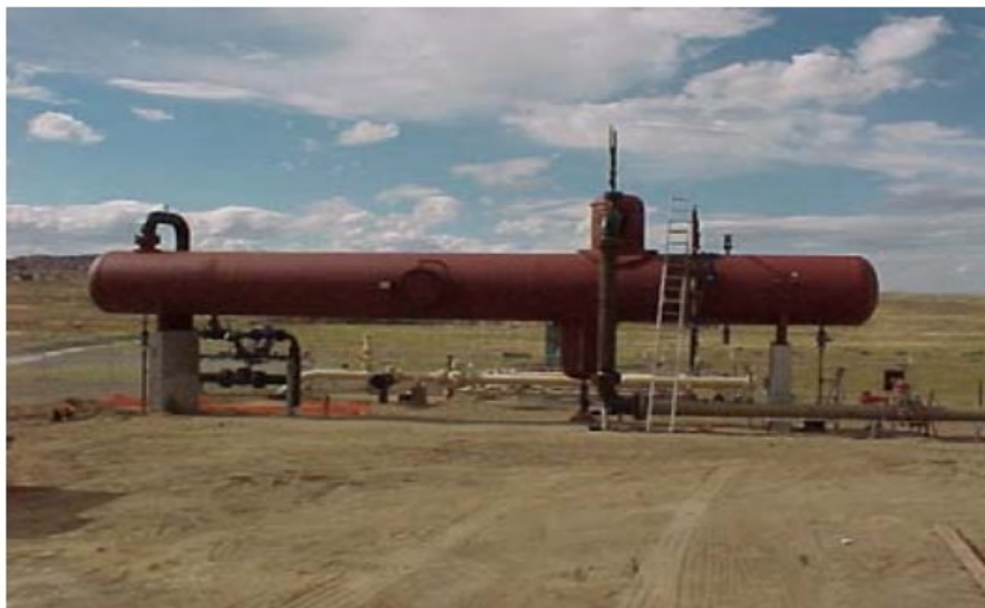
Figure 3-19: An example of a vessel-type slug catcher taken from (Kimmitt et al., 2001)
