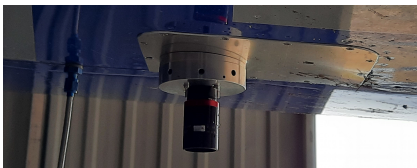
Fig. 3. The modified hyperspectral camera mounted under the left wing using custom aluminium parts.
