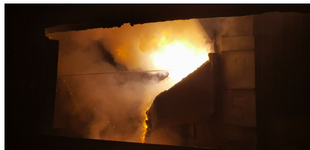
Fig. 3. Tapping at the second taphole.
