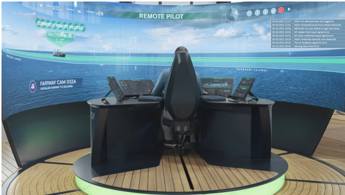
Figure 20: Recommended HMI: Red status indicator (padlock symbol) with alert list that can get shown on demand from the captain.
