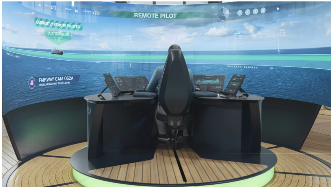
Figure 7: Conceptual remote control stations in the remote operation center. Image taken from Kongsberg Maritime's Youtube video. [6]
