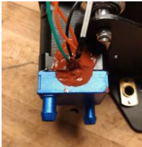
Fig. 41. Mount cooling block and add HTS.
