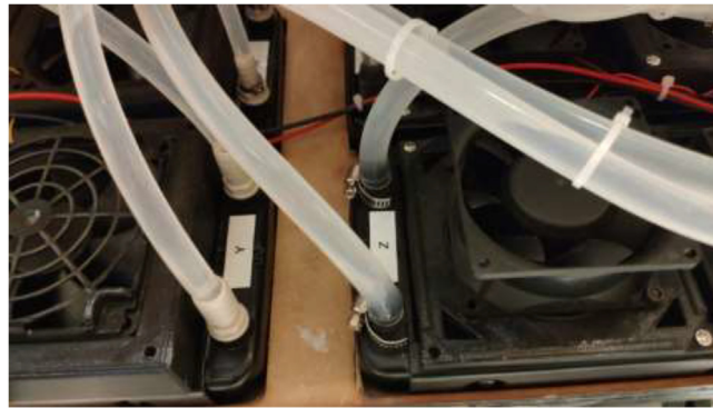
Fig. 103. Tubes installed on radiators.
