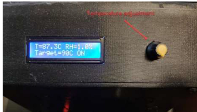
Fig. 134. Drying Chamber control panel.
