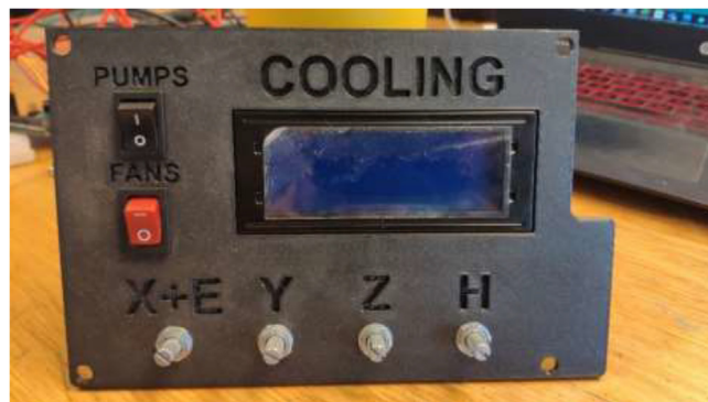
Fig. 92. Cooling cover installation.
