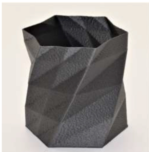
Fig. 139. Vase printed to demonstrate the ability to print larger parts in Z-direction. The height of the item was 100 mm.
