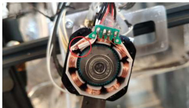
Fig. 39. Inserting thermistor for temperature observation.
