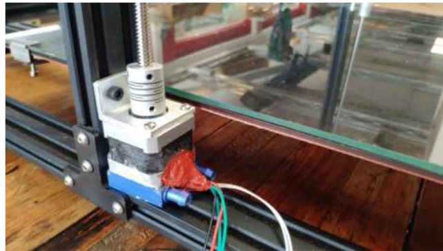
Fig. 53. Upgraded Z motors with new Z motor holder.
