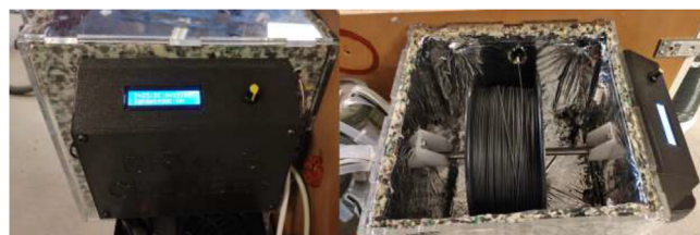
Fig. 125. Finished drying chamber.
