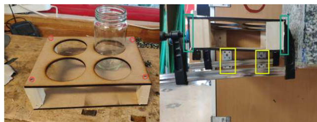
Fig. 23. Reservoir holder. Wood screws (red), angle brackets (yellow), and reservoir holder sides (green). (For interpretation of the references to color in this figure legend, the reader is referred to the web version of this article.)
