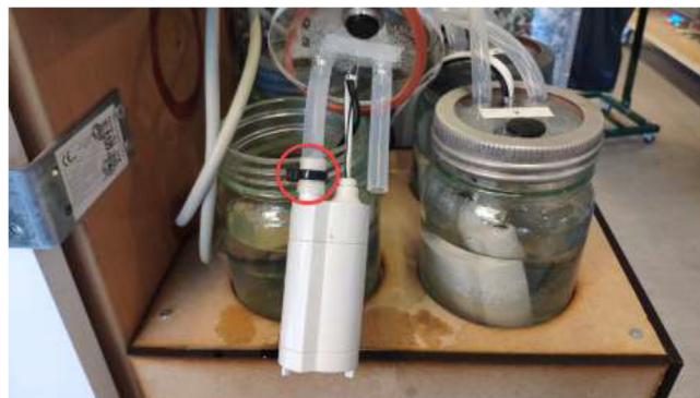
Fig. 98. Tube mounted using zip-tie to pump.
