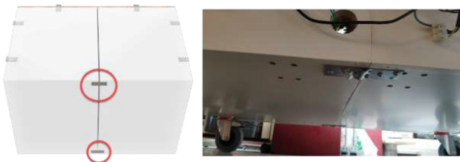
Fig. 5. Interconnection of two closets.
