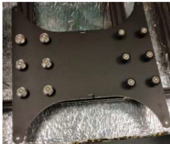
Fig. 47. V-rollers in POM (right) should be replaced with rollers in stainless-steel(left).
