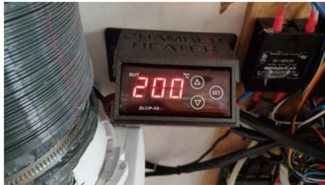
Fig. 131. Integrated PID controller.
