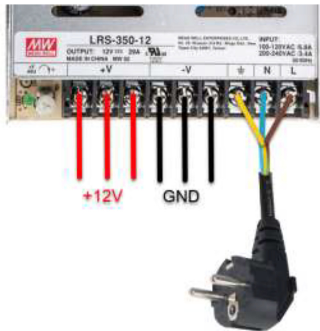
Fig. 78. 3D printer PSU wiring diagram [19,20]
