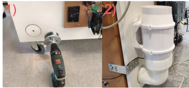
Fig. 20. Exhaust fan mounting steps. 1) Drill a hole for the exhaust. 2) Install fan and printed bracket.
