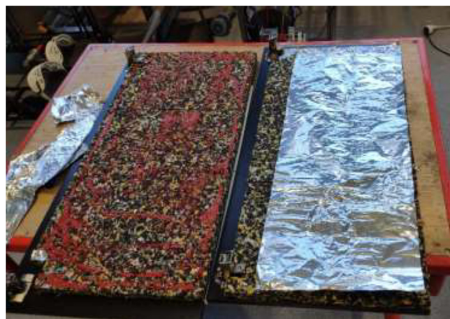
Fig. 14. Optionally, replacing reflective foil with aluminum foil.
