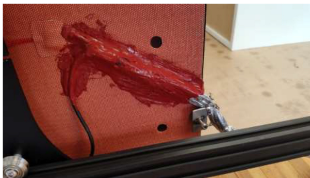
Fig. 66. Strain relief for silicone heater using HTS.
