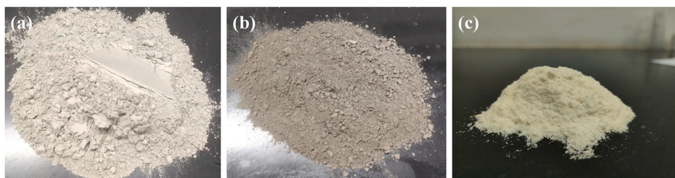
Fig. 2. Multi- source solid wastes: (a) HCFA, (b) SS and (c) sodium sulfate recovered from the waste liquid in chemical fiber industry.
