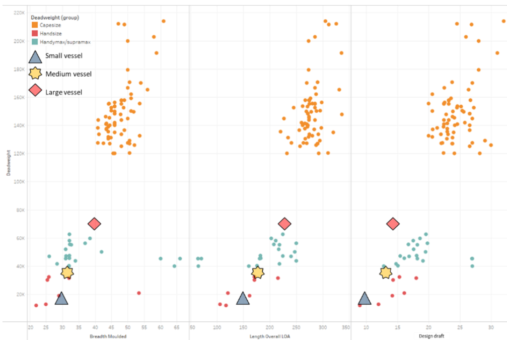
Figure 9: Hull characteristics of vessels compared to various FPSOs. Reference vessel data from IHS Fairplay.
