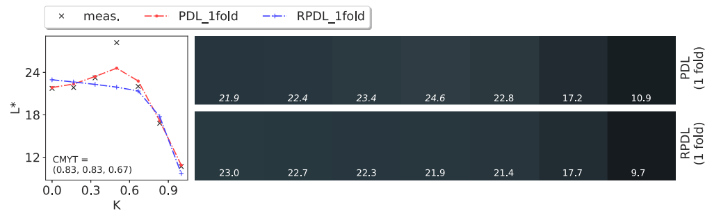
Fig. 1. Lightness L^* as a function of black material K with other materials fixed on a tonal case of the Mimaki 2 dataset (the fixed tonal values are shown at the lower left of the figure), and the resulting colors. The L^* values are shown as white numerical text, with italic font indicating L^* -vs- K monotonicity violations. The PDL/RPDL prediction in this figure is from a single PDL/RPDL model respectively. The figure shows that the training data itself has errors leading to monotonicity violations, and that the PDL model overfits to the erroneous data without considering monotonicity. In contrast, the proposed RPDL model ensures monotonicity despite the data outlier, indicating better robustness against errors in training data.
