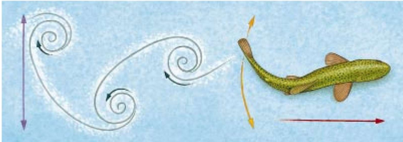
Figure 1-3. The wake of a swimming fish has reverse-von Kármán vortex street, associated with thrust generation (Taken from Triantafyllou and Triantafyllou, 1995)
