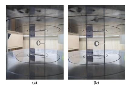
**Figure 2.** Two keyhole notched specimens shown during the compressive fracture test: (a) PMMA,  $\rho = 4$  mm; (b) GPPS,  $\rho = 4$  mm.
