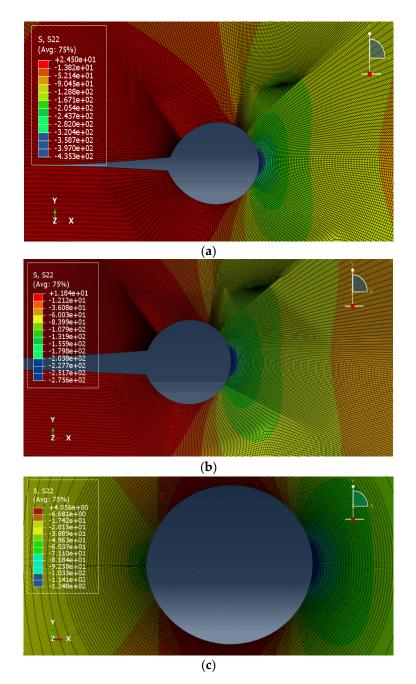
**Figure 9.** Examples of stress distributions (MPa) for keyhole notches: (a) PMMA,  $\rho = 0.5$  mm,  $P_1 = 16636$  N; (b) GPPS,  $\rho = 0.5$  mm,  $P_1 = 7360$  N; (c) GPPS,  $\rho = 4$  mm,  $P_2 = 9186$  N.
