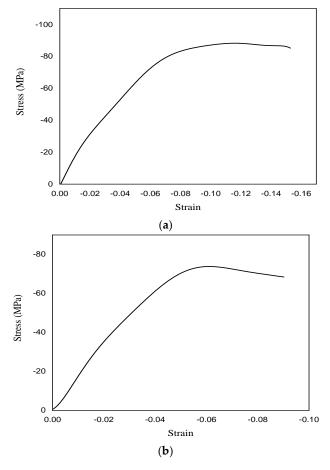
Figure 6. Compressive stress-strain curves for (a) PMMA and (b) GPPS.
