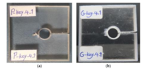
**Figure 7.** Two of the keyhole notched polymeric specimens after the compressive fracture test: (a) PMMA,  $\rho = 4$  mm; (b) GPPS,  $\rho = 4$  mm.
