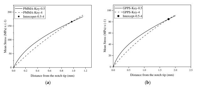
Figure 11. Variations of mean compressive stress versus the distance from the notch tip: (a) PMMA; (b) GPPS.
