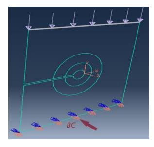
**Figure 4.** Loading and boundary conditions for the keyhole notched specimens subjected to compressive loading. BC: boundary conditions.
