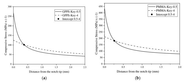
Figure 10. Variations of compressive stress versus the distance from the notch tip: (a) PMMA; (b) GPPS.
