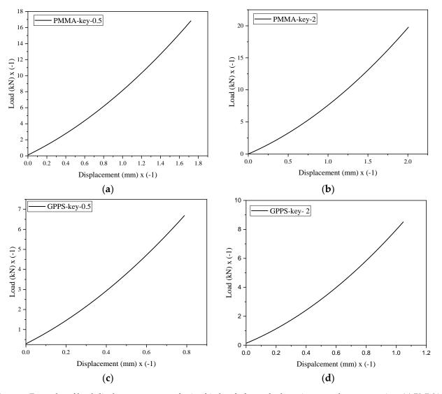
is different from that observed in fracture tests of notched components either under tension or compression. Most probably, this is because of the contact between the key-hole notch parallel faces during loading.
