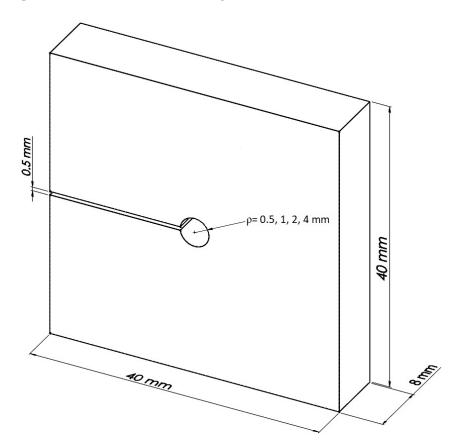
Figure 1. Geometry of the fracture specimens.
