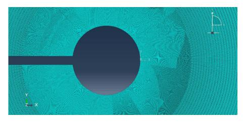
Figure 5. Detail of the mesh pattern around the keyhole notch.
