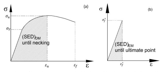
Figure 3. Schematic of the tensile stress-strain curves: (a) real ductile material (DM); (b) equivalent (brittle) material (EM).
