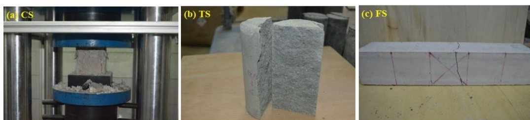
Figure 9. Failure patterns of SCGCs incorporated with 30% FA (a) CS, (b) TS, and (c) FS.
