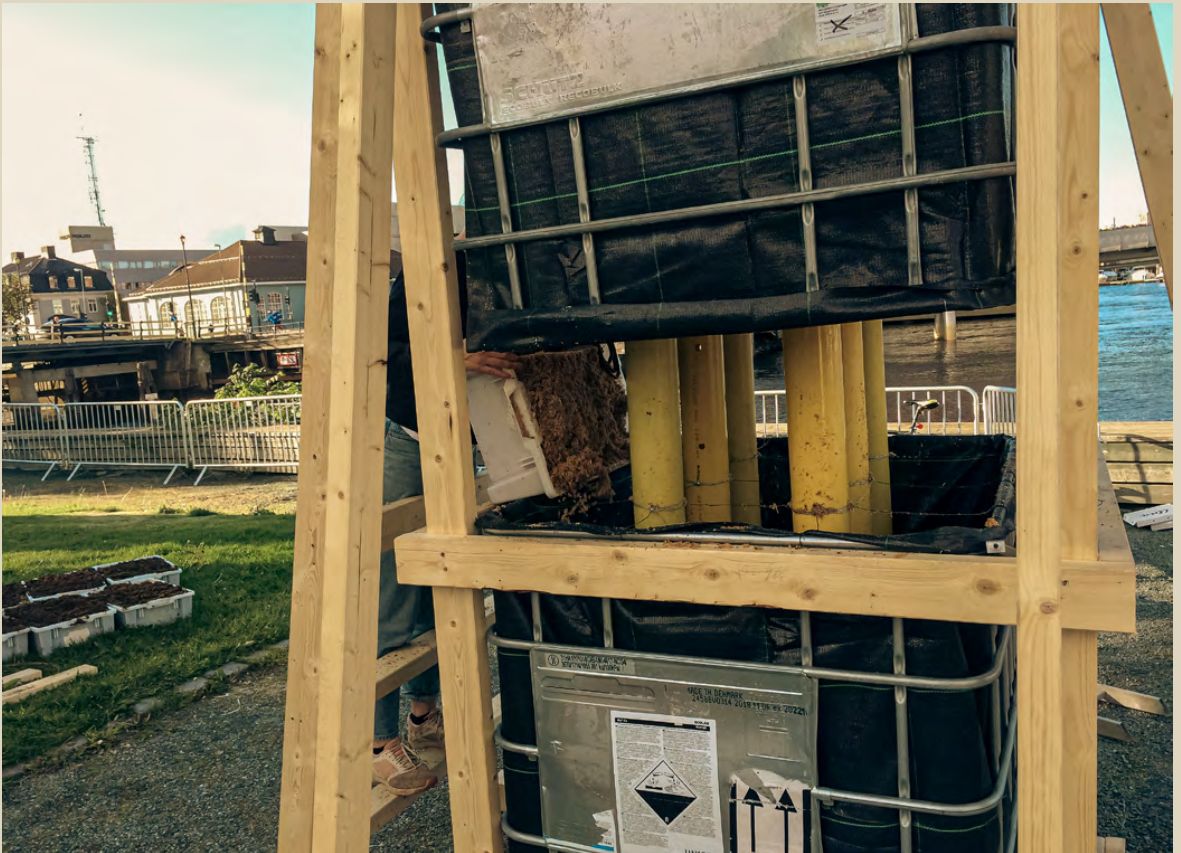
Filling the reactor, with woodchips, coffee shells and spent grain. Pipes are left in the compost for 48 hours and make air channels that allows for aerobic composting.
