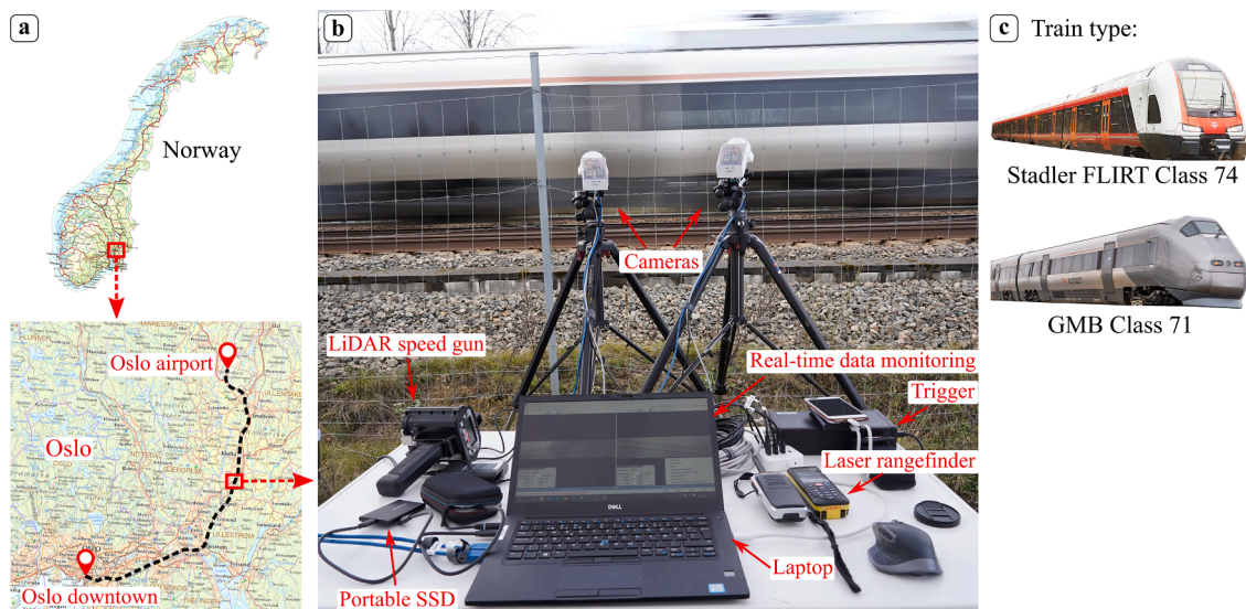
Fig. 7. Overlap span measurement at Oslo airport line. Photography: Tengjiao Jiang/NTNU. Maps courtesy of Kartverket©. Photos of the FLIRT train type courtesy of Norske tog© and the GMB train type courtesy of Flytoget©.
