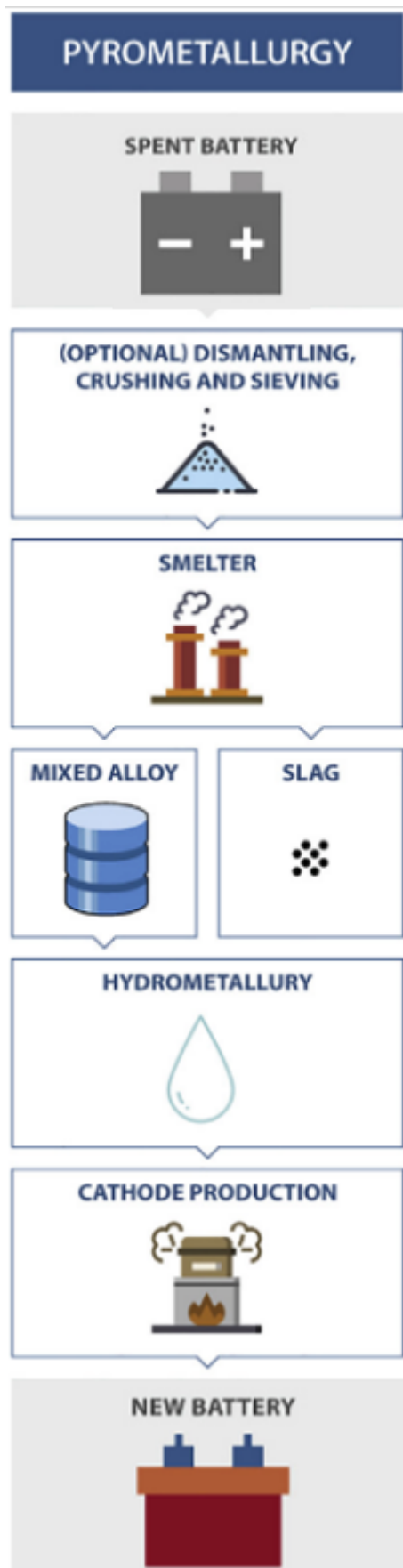
Figure 2.2.2: General flow sheet over the pyrometallurgical process [18].
