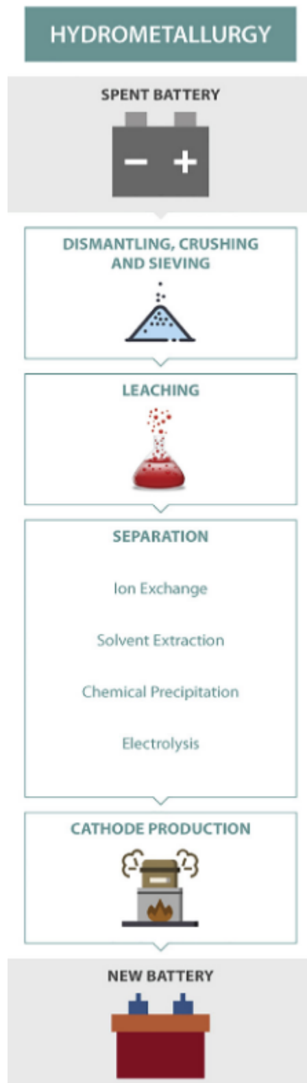
Figure 2.2.3: General flow sheet over the hydrometallurgical process [18].
