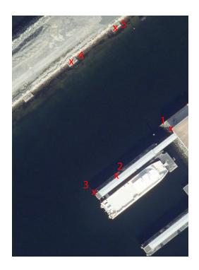
Fig. 2. Docking area seen from above with UWB anchor placement. Courtesy of Google Earth.
