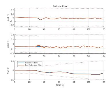
Fig. 15. Estimation error in attitude with UWB bias estimation
