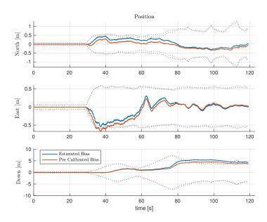
Fig. 14. Estimation error in position with UWB bias estimation
