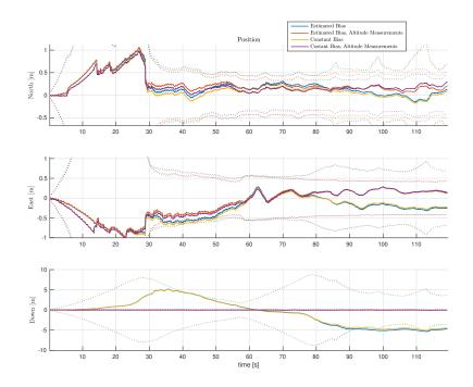
Fig. 18. Estimation error in position with virtual altitude measurement in dataset 2
