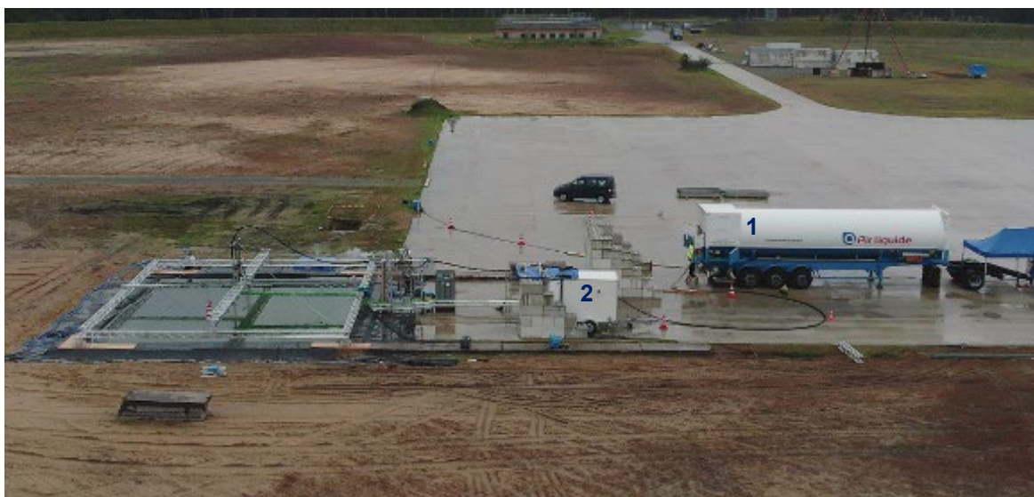
Figure 1: View of the test set-up to study the release of LH 2 onto and under water. The picture shows the basin on the left with a bridge structure for holding the release mechanism and instrumentation. On the right the trailer, 1, carrying the LH 2 and the cabin, 2, used for logging equipment.
