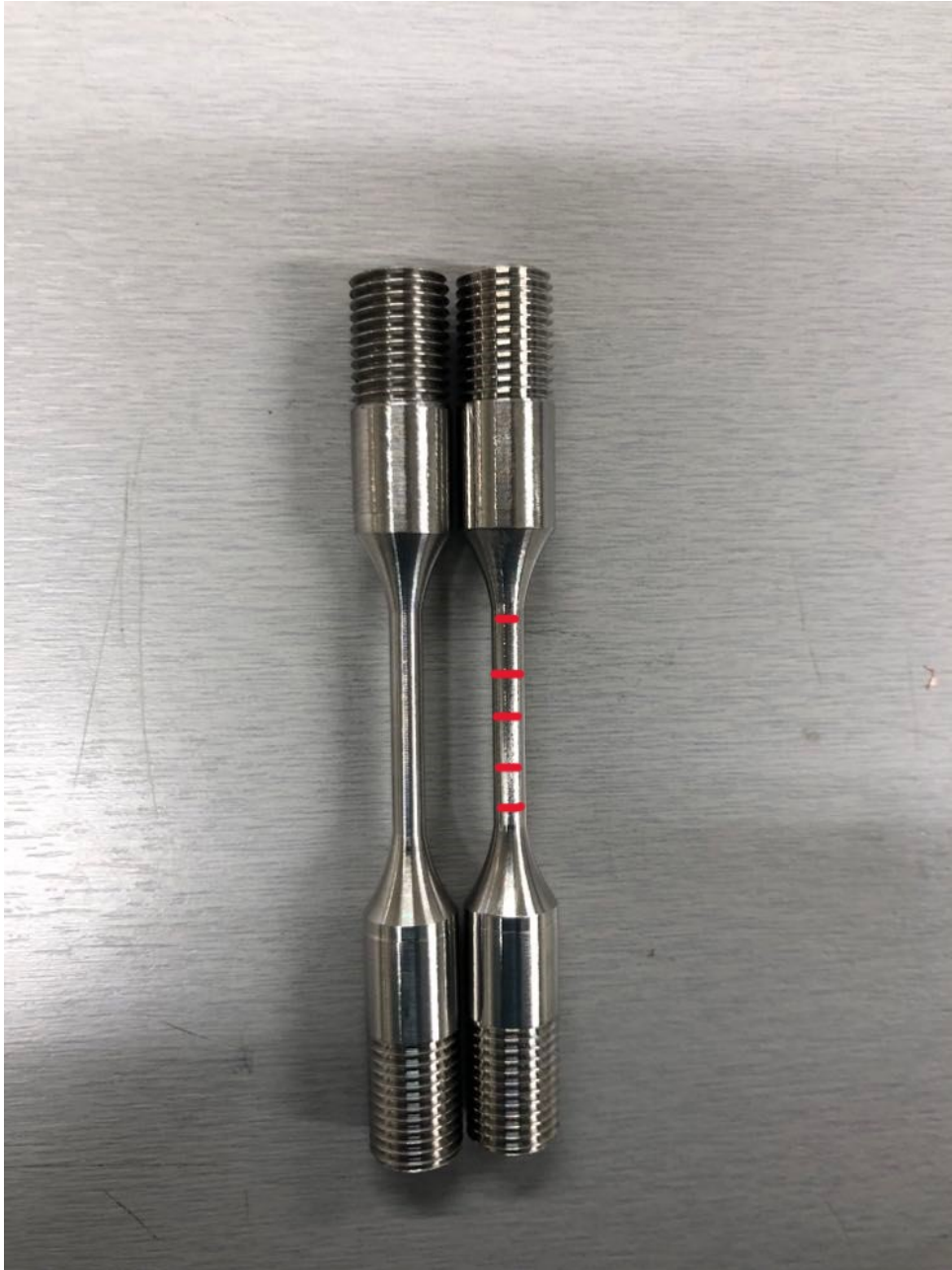
Figure 3.3.3: Image of two milled and test ready specimens for HISC testing.
