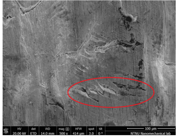
(b) Secondary crack in marked area.
