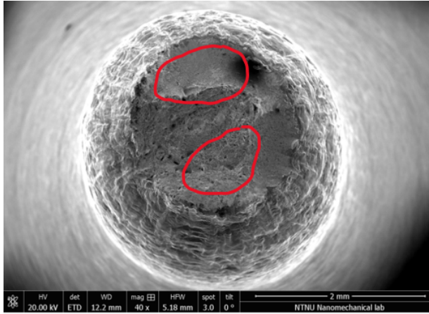
(a) Overview of fracture surface.
