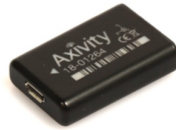
Figure 3.1: The Axivity AX3 accelerometer
