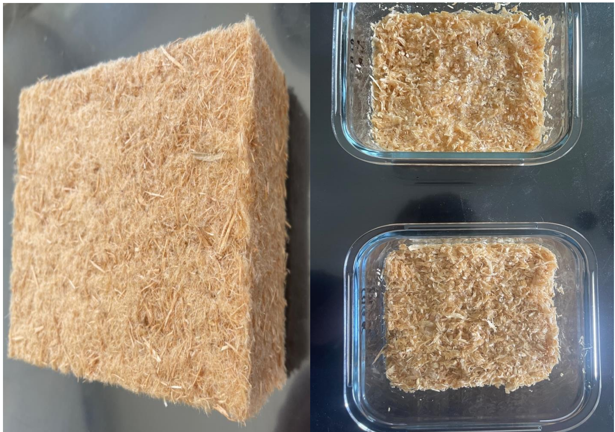
Picture 9 and 10. Comparing picture of original wood fiber insulation and PVA-based wood fiber.
