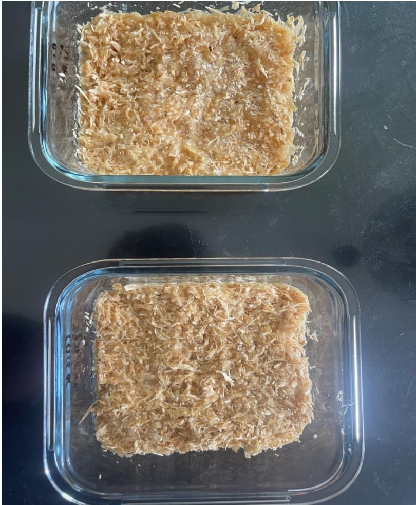
Picture 6. Specimens after heating and 48 hours curing. The Oven heated specimen showed the highest similarity to the original wood fiber insulation.
