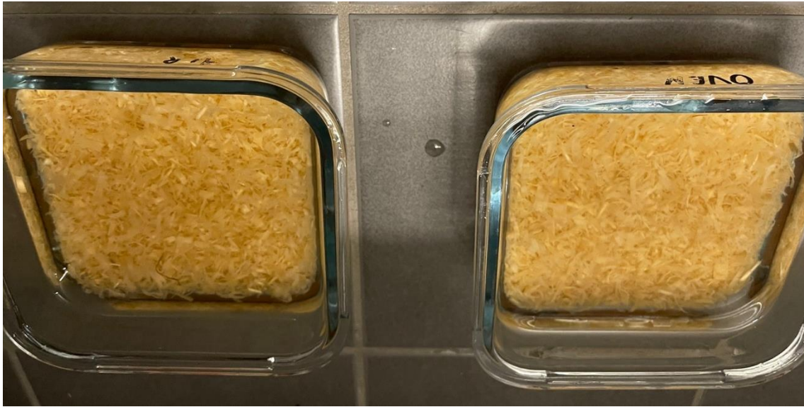
Picture 8. Picture of the wood fiber in PVA taken out of the bath.
