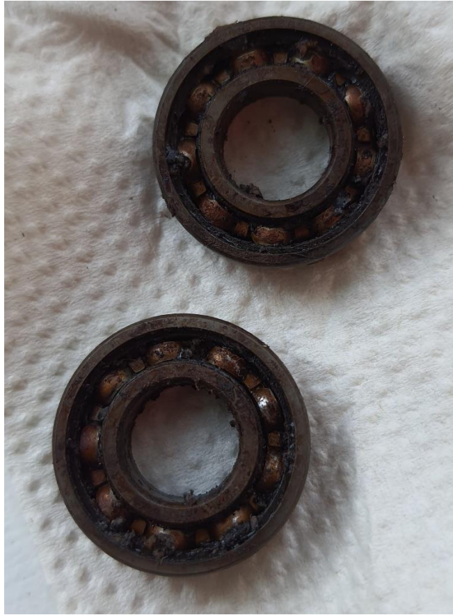
FIGURE 21 RESULTING RUSTED BEARINGS
