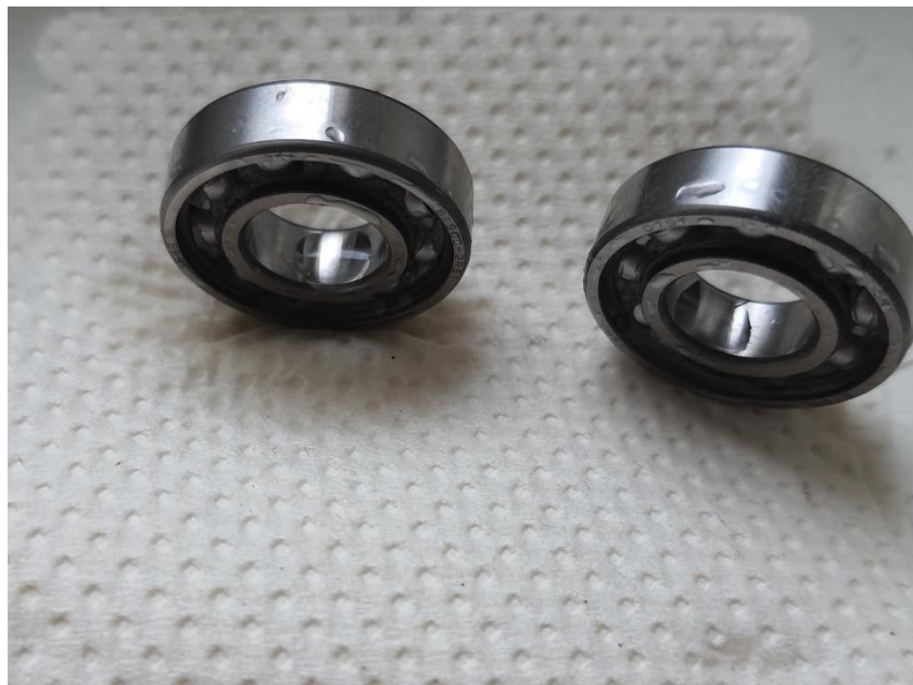
FIGURE 20 VINEGAR COVERED BEARINGS SET TO DRY
