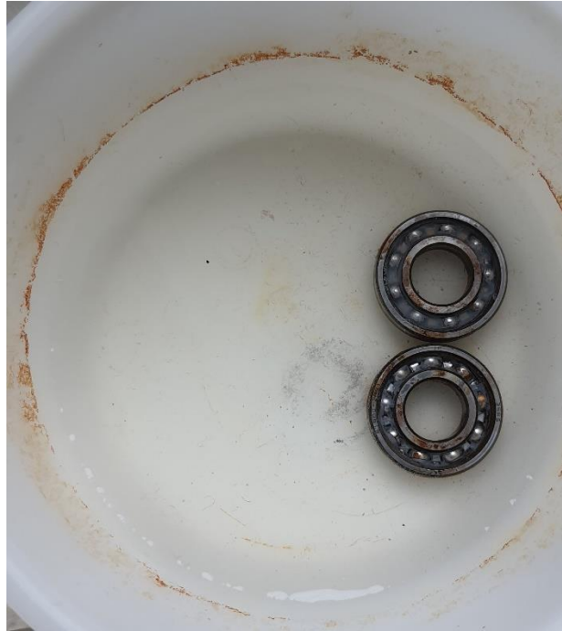
FIGURE 19 BEARINGS SUBMERGED IN VINEGAR
