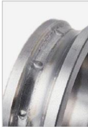
FIGURE 5 INDENTATION (BRINELLING) ON BEARING RACEWAY. (LANGNAU, 2013)
