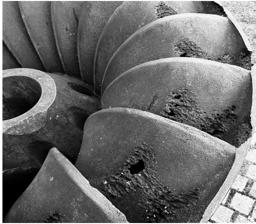
Figure 2.9: Francis runner blades subjected to notable cavitation damage.
