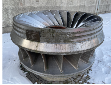
(b) A replica of the Francis runner from Bratsberg hydropower plant.
