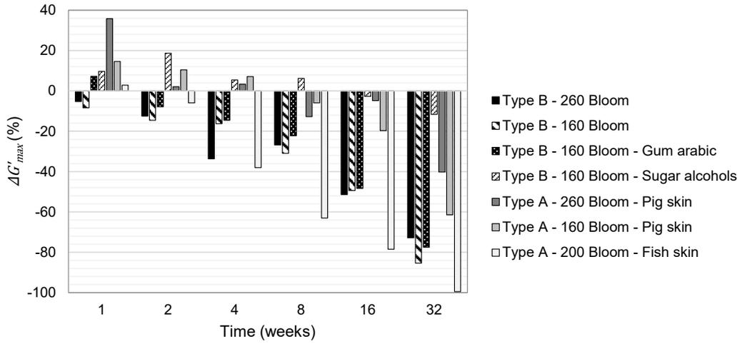
Supplementary Figure 4: The change in  $G'_{max}$  after storage at 30 °C for 32 weeks. The  $\Delta G'_{max}$  is given as percent change compared its  $t_0$  value for each gel.
