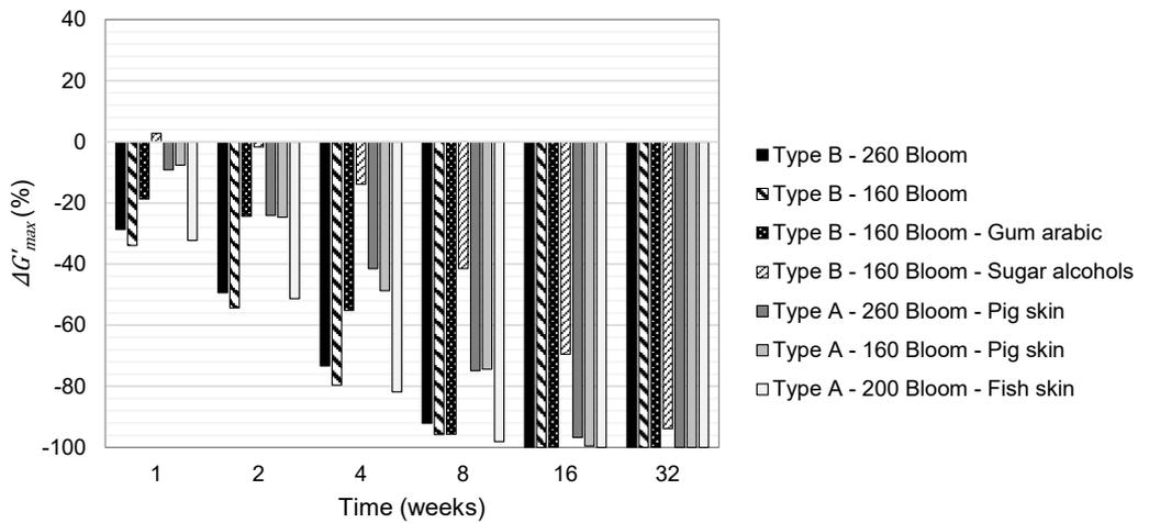
Supplementary Figure 5: The change in  $G'_{max}$  after storage at 40 °C for 32 weeks. The  $\Delta G'_{max}$  is given as percent change compared its  $t_0$  value for each gel.
