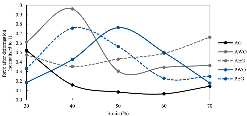
Supplementary Figure 4: Force after gel deformation at strains from 30 to 70%. The maximum force at single compression was regarded as 1 and force after deformation was normalized to 1. The abbreviations and compositions of the gels are given in Table 1.
