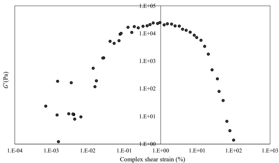
Supplementary Figure 1: Strain sweep of 7.15% agar gel (AG).
