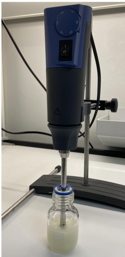
*Figure 12: Photograph of IKA® T10 basic Ultra-Turraz®, one of the high-speed mixer homogenizers used in this work.*
