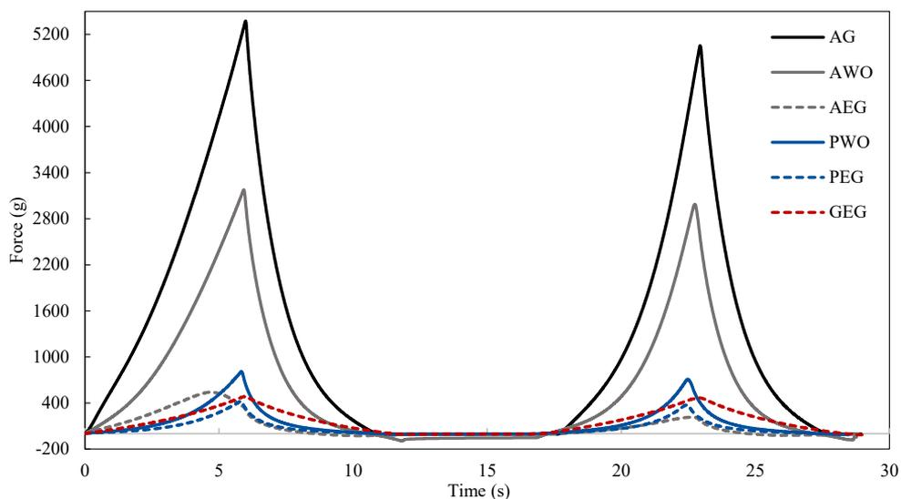
Supplementary Figure 2: Texture profile analysis of the gels with 30% strain. Each curve represents the average of 7-10 gels (obtained from a single batch). The abbreviations and compositions of the gels are given in Table 1.
