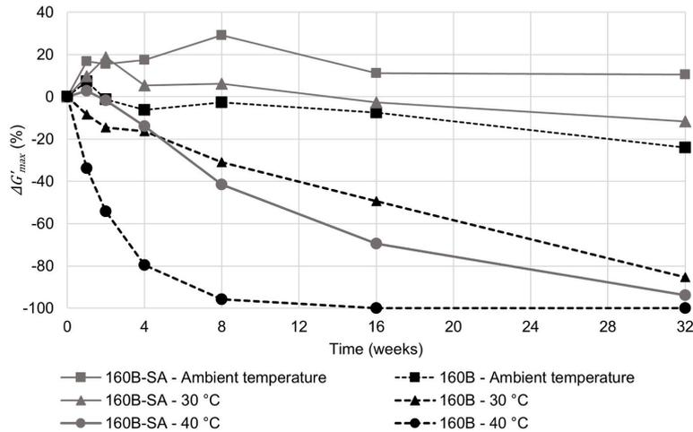
**Fig. 1.** The change in  $G'_{max}$  of type B – 160 Bloom gelatin gel with (gray, 160B-SA) and without (black, 160B) sugar alcohols (23 (w/w)% sorbitol and 35.2 (w/w)% xylitol) over 32 weeks of storage. The  $\Delta G'_{max}$  is given as percent change compared to its  $t_0$  value. Different storage temperatures are shown as: (■) ambient temperature, (▲) 30 °C, and (●) 40 °C. The data points are connected to guide the eye.
