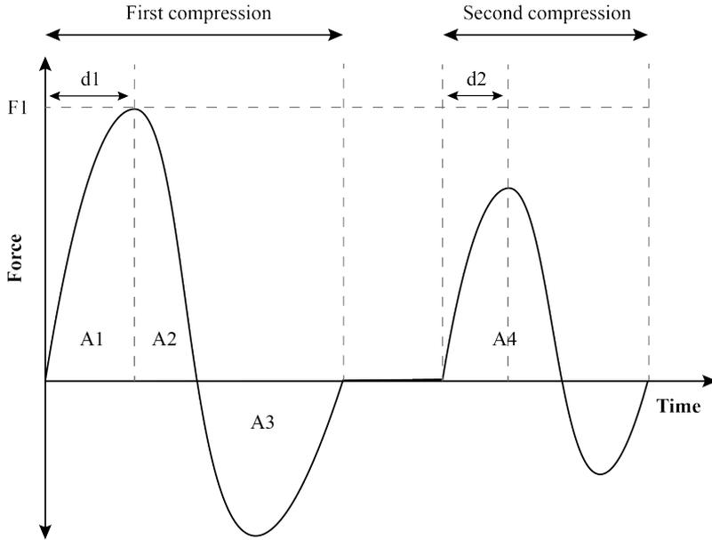
Figure 11: A typical texture profile analysis curve.
