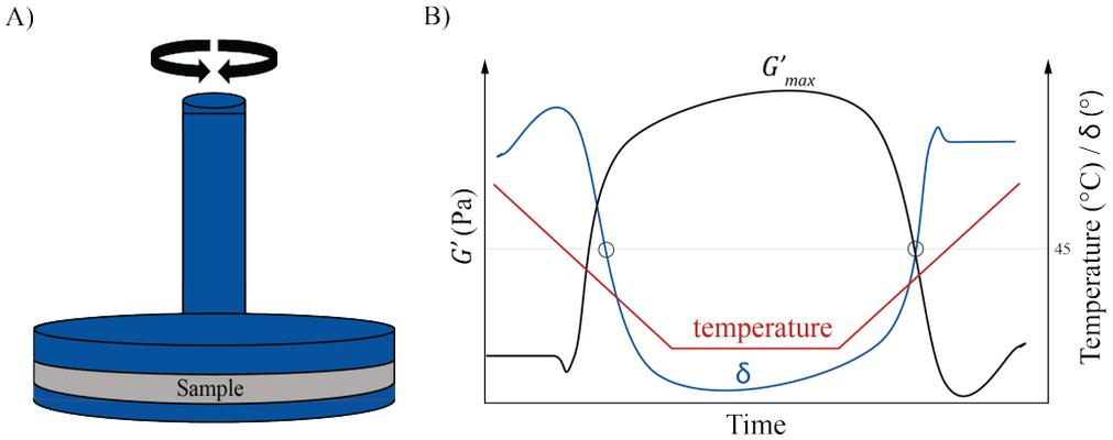
Figure 9: A) Schematic representation of an oscillatory measurement setup. B) An example curve from a small amplitude oscillatory shear measurement showing how shear modulus ( $G'$ ) and phase angle ( $\delta$ ) for the sample changes with temperature.
