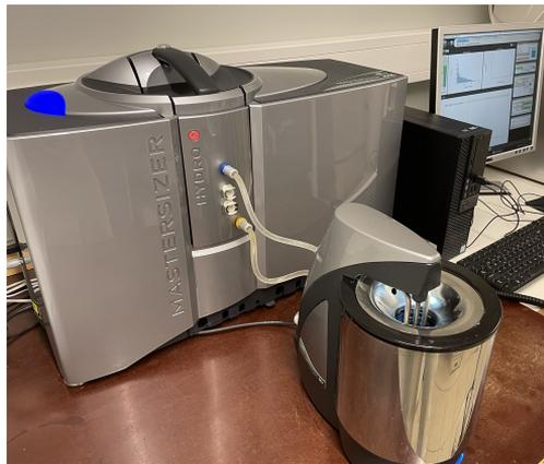
Figure 15: Photograph of the Malvern Mastersizer Hydro®3000 that was utilized for laser diffraction particle analyses in the present work.
