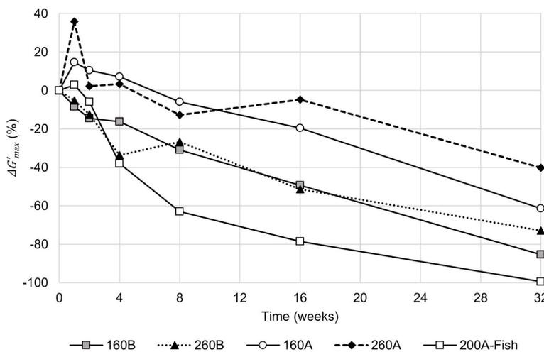
Fig. 3. The change in  $G'_{max}$  of gelatin gels from three different sources over 32 weeks storage at 30 °C. Two different Bloom strength type B and type A – pig skin gelatins are shown. The  $\Delta G'_{max}$  is given as percent change compared to its  $t_0$  value. The data points are connected to guide the eye.
