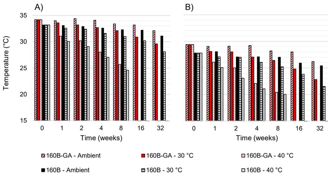
Supplementary Figure 2: A) Melting temperature ( $T_m$ ) and B) gelling temperature ( $T_g$ ) of type B – 160 Bloom gelatin gel with (160B-GA) and without (160B) gum arabic over 32 weeks storage at ambient temperature, 30 °C or 40 °C. Empty bars at week 16 and 32 indicate too low  $G'$  values to detect a temperature corresponding to 45° phase angle.
