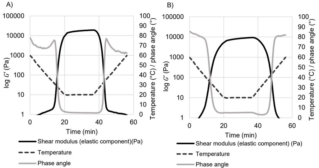
Supplementary Figure 6: Small amplitude oscillatory shear measurements of A) 160B and B) 160B-SA after one week storage at ambient temperature.
