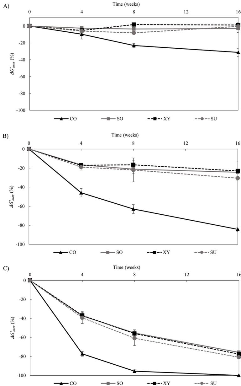
**Fig. 1.**  $\Delta G'_{max}$  of fish gelatin gels with different non-reducing sugars (52 (w/w)%) during storage at A) ambient temperature, B) 30 °C, and C) 40 °C up to 16 weeks. The  $G'_{max}$  values are the average of independent replicates (three for CO, and two for SO, XY, and SU), and the error bars indicate standard deviation. The data points are connected to guide the eye. The abbreviations and compositions of the gels are given in Table 1.
