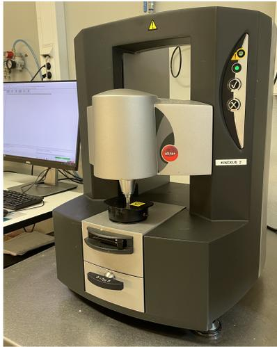
Figure 7: Photograph of Malvern Kinexus ultra+, the rheometer used in the present work.
