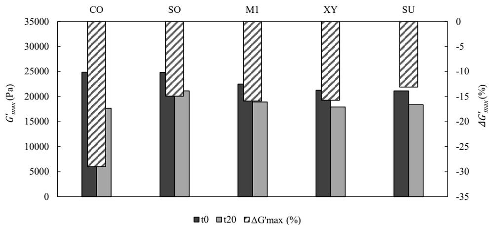
Supplementary Figure 1: Short-term stability test of fish gelatin gels with different co-solutes. The change in  $G'_{max}$  after the short-term stability test at 55 °C for 20 hours ( $t_{20}$ ) are shown.  $\Delta G'_{max}$  indicates percent change compared to the gels  $t_0$  value. The abbreviations and compositions of the gels are given in Table 1.
