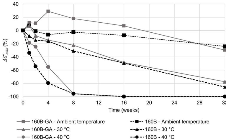
Fig. 2. The change in  $G'_{max}$  of type B – 160 Bloom gelatin gel with (gray, 160B-GA) and without (black, 160B) gum arabic (4 (w/w)%) over time. The  $\Delta G'_{max}$  is given as percent change compared to its  $t_0$  value. Different storage temperatures are shown as: (■) ambient temperature, (▲) 30 °C, and (●) 40 °C. The data points are connected to guide the eye.
