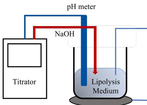
Figure 18: A schematic representation of the *in vitro* lipolysis set up used in this project.
