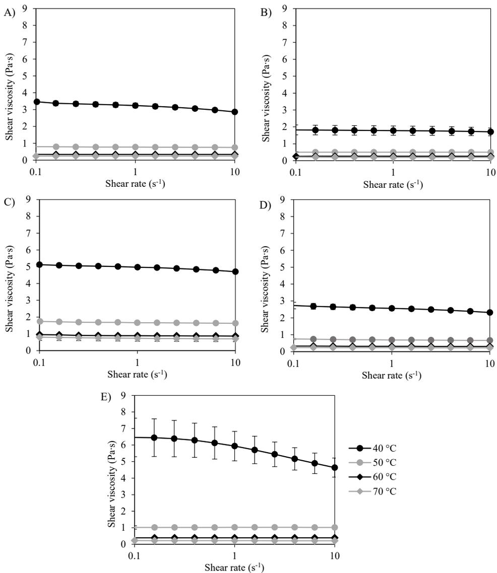
Supplementary Figure 7: Viscosity sweep of A) SO, B) XY, C) SU, D) M1, and E) M2 at 40, 50, 60, and 70 °C. The abbreviations and compositions of the gels are given in Table 1.
