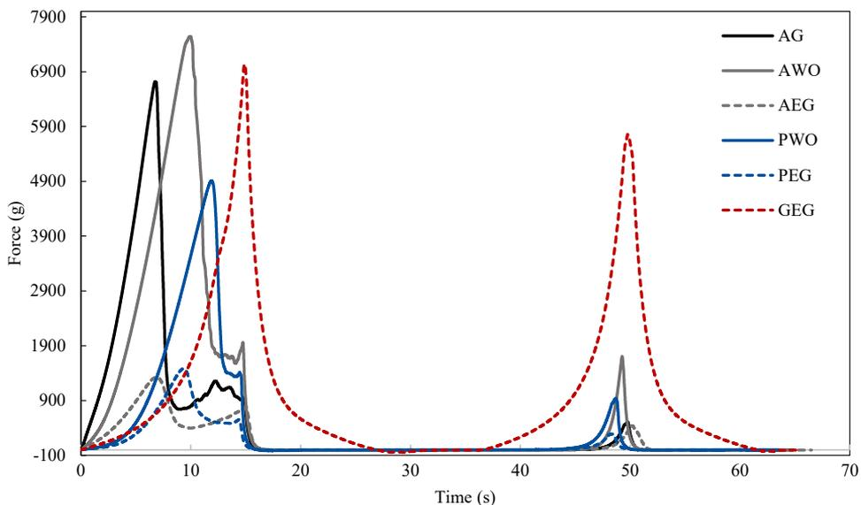
Supplementary Figure 3: Texture profile analysis of the gels with 75% strain. Each curve represents the average of 7-10 gels (obtained from a single batch). The abbreviations and compositions of the gels are given in Table 1.
