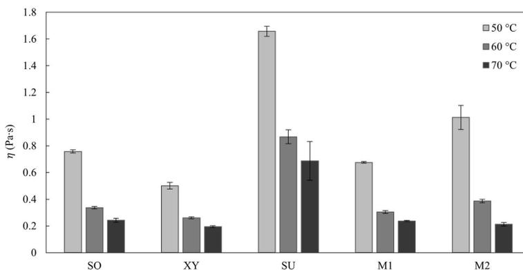
**Fig. 6.** Shear viscosity ( $\eta$ ) of fish gelatin gels with different co-solutes at 1 s<sup>-1</sup> shear rate. The data is given as the average of two replicate gels and the error bars show the standard deviation. The abbreviations and compositions of the gels are given in Table 1.
