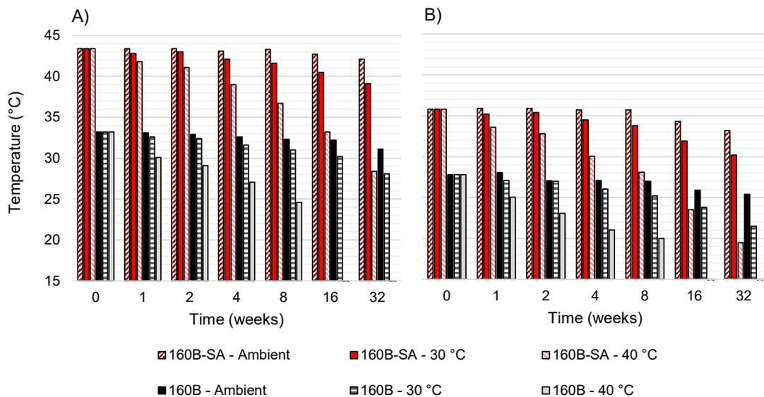
Supplementary Figure 1: A) Melting temperature ( $T_m$ ) and B) gelling temperature ( $T_g$ ) of type B – 160 Bloom gelatin gel with (160B-SA) and without (160B) sugar alcohols over 32 weeks storage at ambient temperature, 30 °C or 40 °C. Empty bars at week 16 and 32 indicate too low  $G'$  values to detect a temperature corresponding to 45° phase angle.
