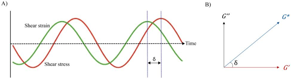
Figure 8: A) Sinusoidal curves of shear stress and shear strain. Modified from Chandran et al. 2020. B) The trigonometric relationship between complex modulus ( $G^*$ ), dynamic storage modulus ( $G'$ ), dynamic loss modulus ( $G''$ ), and phase angle ( $\delta$ ).
