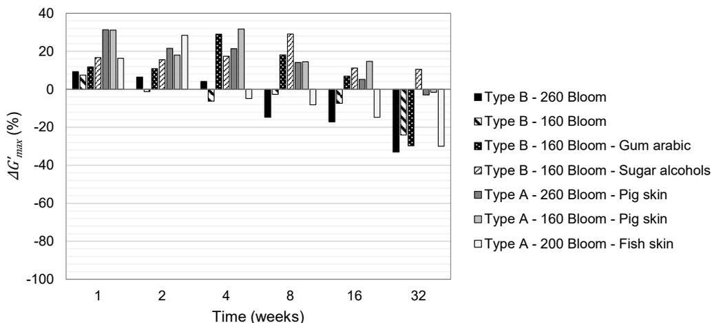
Supplementary Figure 3: The change in  $G'_{max}$  after storage of different gelatin gels at ambient temperature for 32 weeks. The  $\Delta G'_{max}$  is given as percent change compared its  $t_0$  value for each gel.
