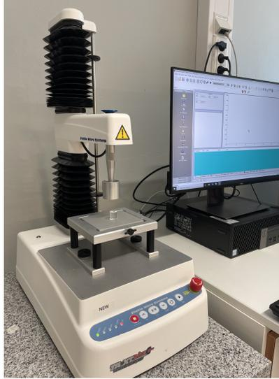
Figure 10: Photograph of Stable Micro Systems Ltd. TA.XT plusC Texture Analyser, used in the present work.
