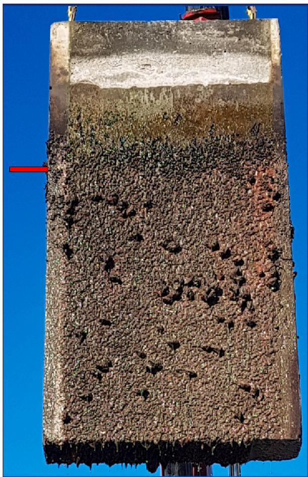
Fig. 4. Visual appearance of an entire concrete panel right after lifting out of the water. The part below mean sea level (red line, 1.3 m from the bottom) is covered with barnacles and mussels, the upper approx. 0.35 m is dry, and in between is a gradual transition from heavy to light organic growth. (For interpretation of the references to colour in this figure legend, the reader is referred to the Web version of this article.)
