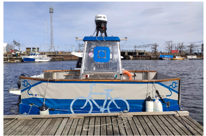
Fig. 1. milliAmpere , an autonomous ferry research platform.
